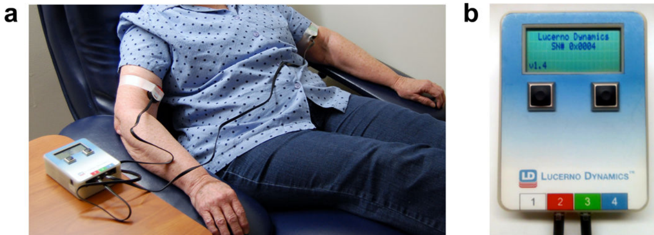
Fig. 1. (a) Sensors containing scintillation material convert gamma radiation, emitted from the decay of ^{18}\text{F} -FDG, to visible light in the form of photon counts/sec. For recordings of the injection arm and control arm, sensors are positioned over the bicep, since the convex shape of the antecubital fossa hinders direct recording from this region. Sensors are held in place using standard medical tape. (b) Sensors are connected via cable to a portable reader module that actively records activity counts at 1-second intervals. Data from each sensor channel (up to four) are digitized, tabulated and exported from the reader in a variety of formats for further computational analysis.
