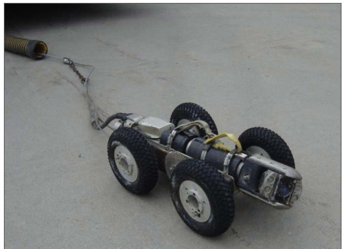
Sewer inspection camera used to find conveyance system failures (lincoln.ne.gov)
