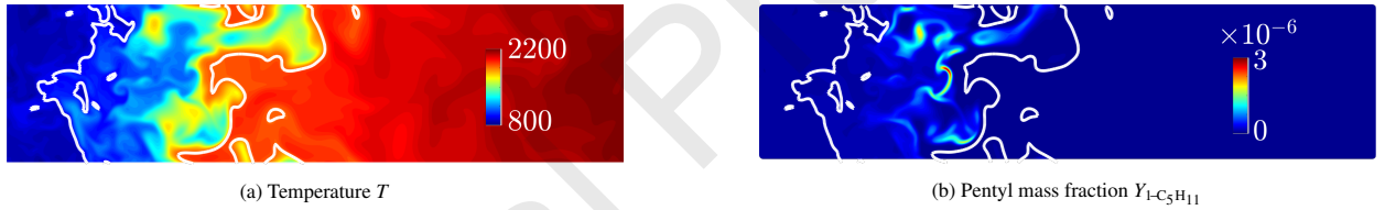
Fig. 9: Two-dimensional slices showing isocontours for the turbulent case ( \Delta t = 10^{-8} s). Two temperature isolines are superimposed in white ( T = 1000 K and T = 1900 K).
