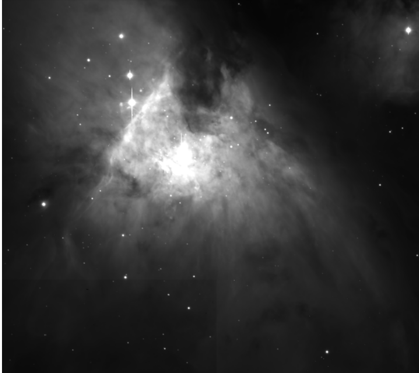
Fig. 25. M42 Nebula taken at the Palomar Observatory during an engineering run on November 2017. Bi-clocking is implemented and no tails are seen behind over illuminated stars.
