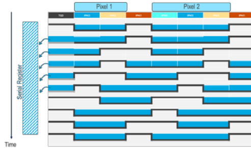
Fig. 9. New waveform proposed to fix the Downing Dip assuming that the last node is missing.
