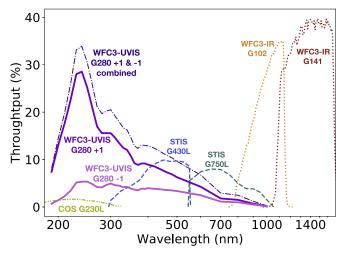
**Figure 1.** Throughput curves for *HST* instruments and modes commonly used for exoplanet time-series observations. Solid lines are the WFC3-UVIS G280 grism orders +1 and -1; the dark dotted–dashed line is the combined transmission of both orders. Dashed lines are STIS G430L and G750L gratings. The -..- line shows the COS G230L. Dotted lines are WFC3-IR G102 and G141 grisms.
