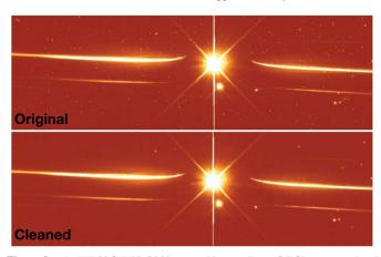
**Figure 3.** *HST* WFC3/UVIS G280 spectral image. Top: "flt" file processed and available on the MAST archive. Bottom: cleaned file with cosmic rays and hot pixels removed, and flat-fielding applied. In this comparison one can clearly see the difference between the original and cleaned data, demonstrating the requirement for accurate and precise treatment of detector artifacts and cosmic-ray hits.
