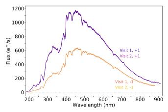
Figure 5. The 16-84 percentile range of the spectral trace of each visit and each order. The +1 orders and -1 orders overlap closely, making it difficult to tell the two visits apart and demonstrating the stability of the instrument and the star. The -1 orders are  $\sim 50\%$  dimmer than the +1 orders, with little to no flux short of 250 nm. Beyond 800 nm fringing patterns can clearly be seen in the stellar spectra and we do not use these wavelengths for the light-curve analysis.
