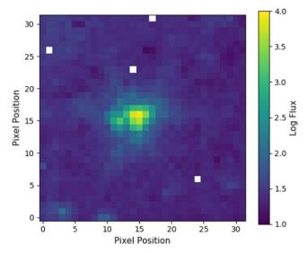
**Figure 7.** Mean flux in *Spitzer*'s 3.6  $\mu$ m channel. Plotting on a logarithmic scale reveals HAT-P-41's faint, nearby companion at pixel position (12, 15). We limit our photometry aperture size to 2.25 pixels to minimize contamination from the companion. Bad pixels are masked in white.
