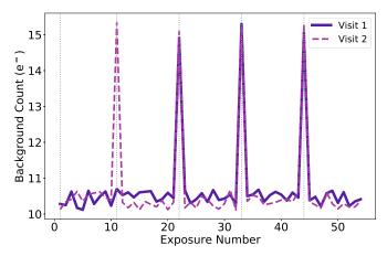
**Figure 2.** Modal background count for each exposure in visit 1 (solid) and visit 2 (dashed) across the whole subarray. The dotted vertical lines indicate the start of a new *HST* orbit. The background is higher at the start of each *HST* orbit with a bimodal distribution, perhaps due to stray earthshine or orbital effects on the telescope.
