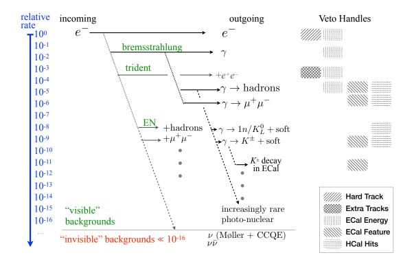
FIG. 5: Flow of important (veto design driving) potential background processes and their raw rates relative to the number of beam electrons incident on the target, shown for a 4 GeV electron beam energy. On the right is a visual summary of which detector systems have significant detection and rejection power for each class of background. Not all reactions considered in our study are explicitly listed in the figure.
