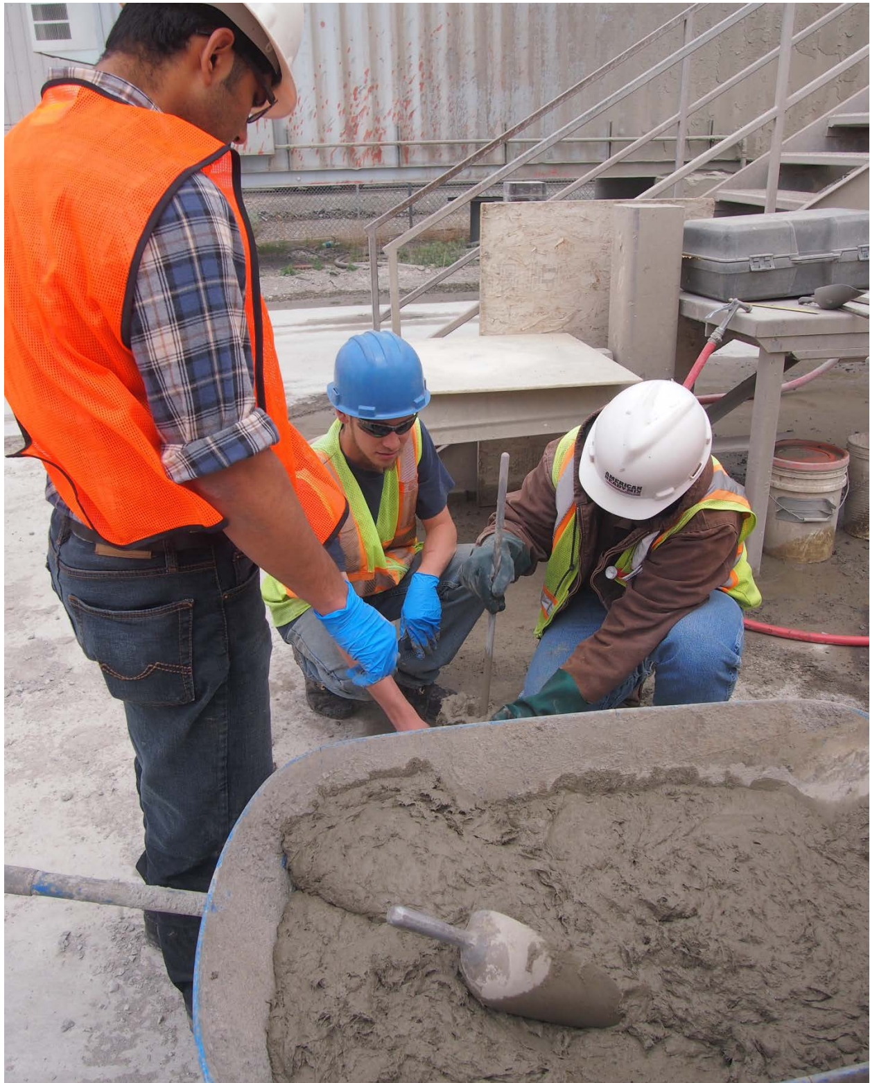
Figure 68 MECC Material from Trial Batch A after Mixing and Discharge from Concrete Truck.
