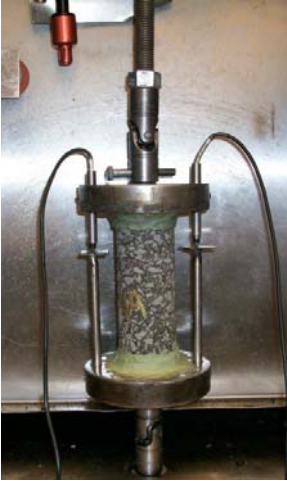
Figure 9. Components of TSRST test and typical stress-temperature curves for HMA mixes
