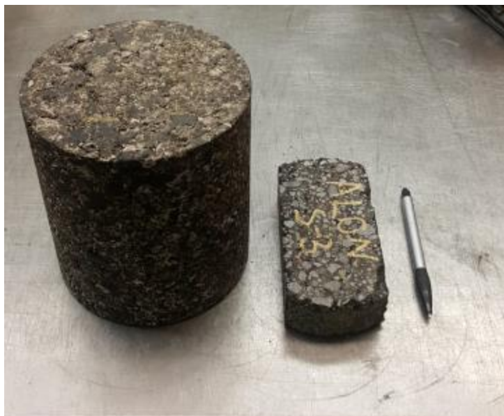
Figure 17. Laboratory molded specimen (left) and trimmed specimen (right).
