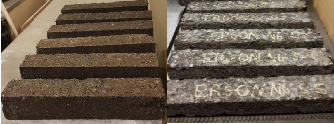
Figure 30. Laboratory compacted specimens (left) and trimmed specimens (right).
