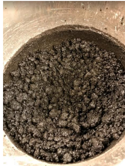
d) RAP + 1.5% Water + LS + Emulsion
