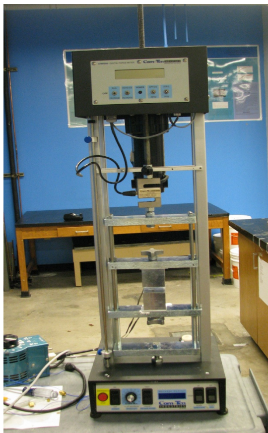
Figure 14: Com Ten tensile testing device used to make MEA
