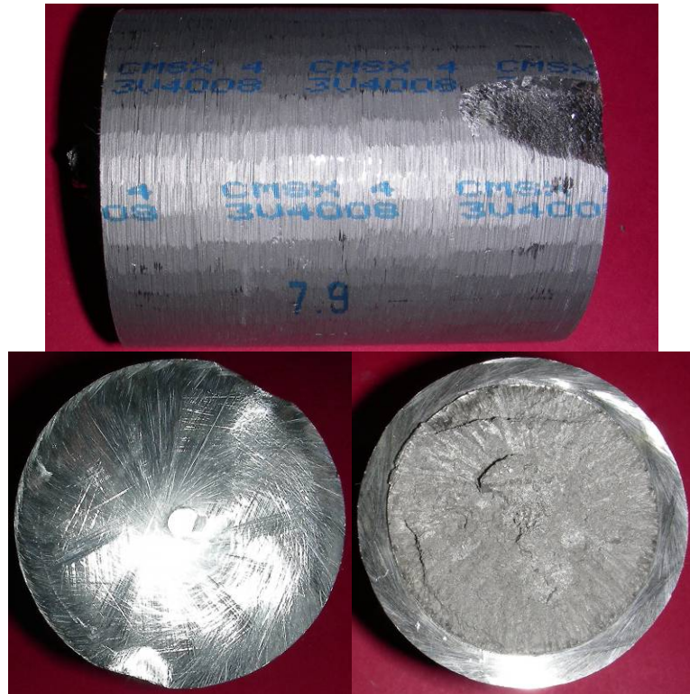
Figure 4. Charge (Ingot) for melting operation of CMSX-4 castings
