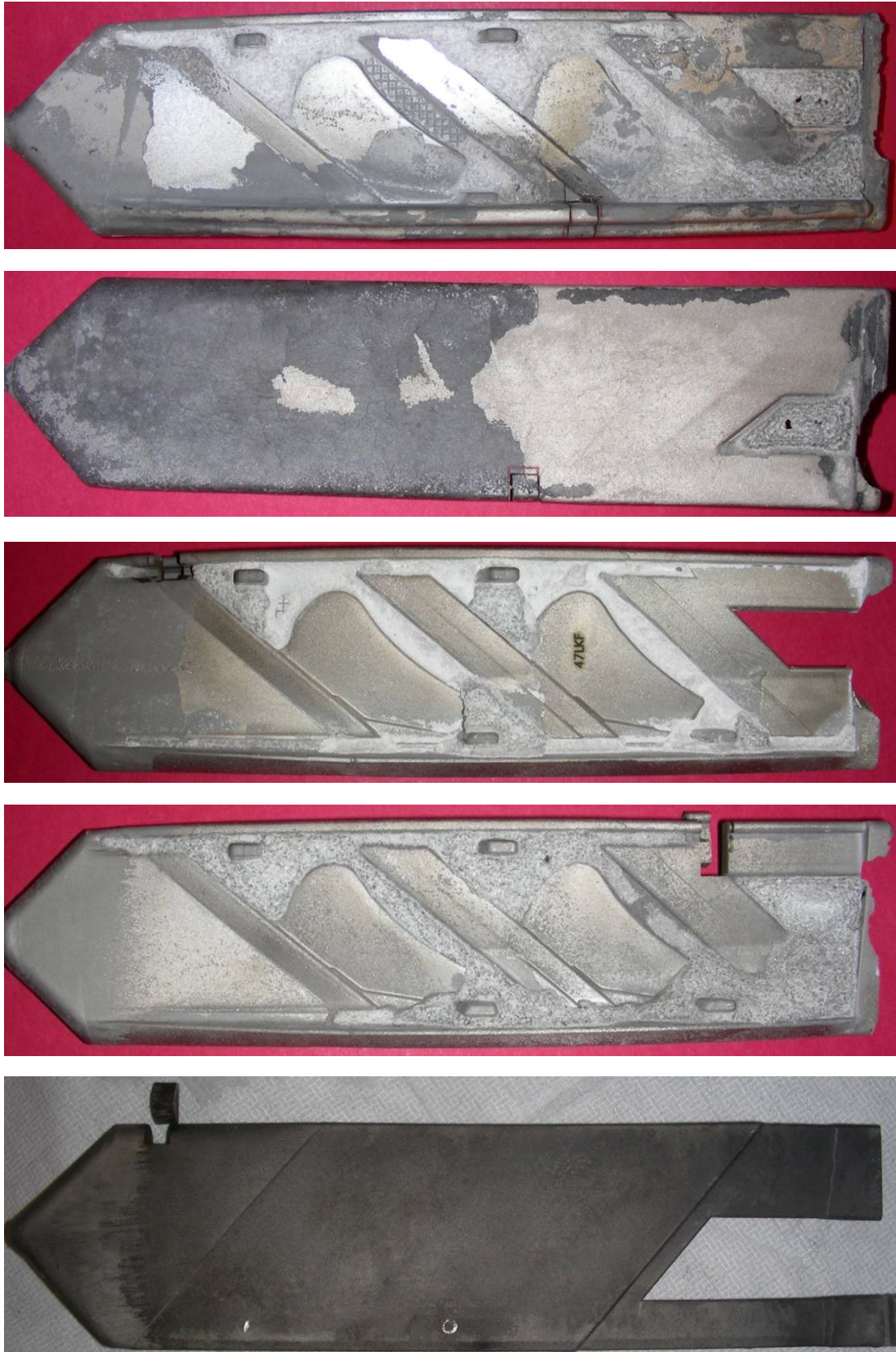
Figure 32. a) Samples (1-5) sectioning for surface characterization
