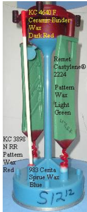
Figure 5. A typical wax pattern assembly of CMSX-4 single crystal castings
