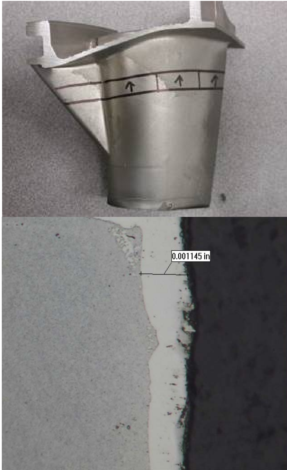
Figure 22.a) A typical metal mold reaction layer on the CMSX-4 airfoil casting
