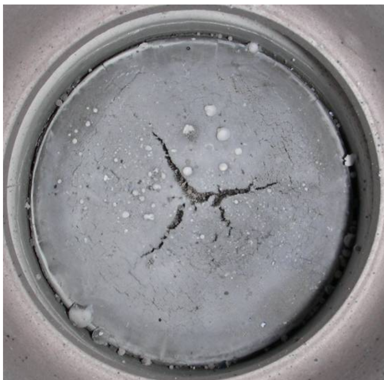
Figure 47. b) more dross on the surface of pouring basin of CMSX-4 casting with secondary grain defect
