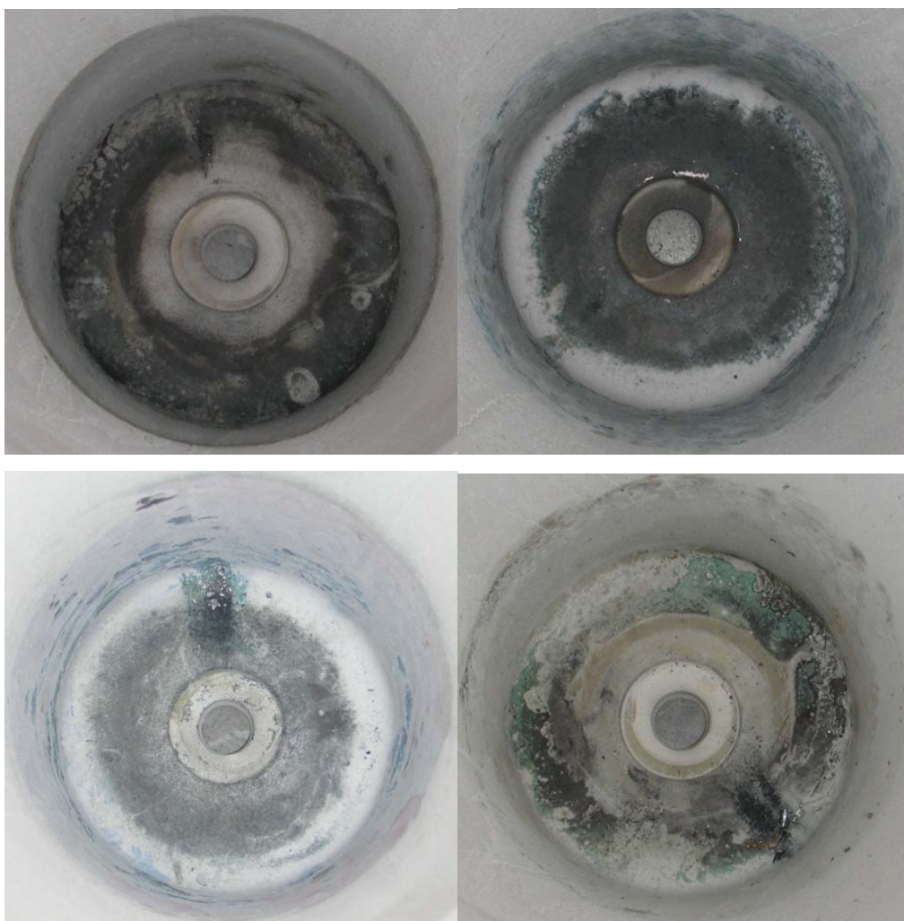
Figure 132. Alumina crucibles were wetted by CMSX-4 melt
