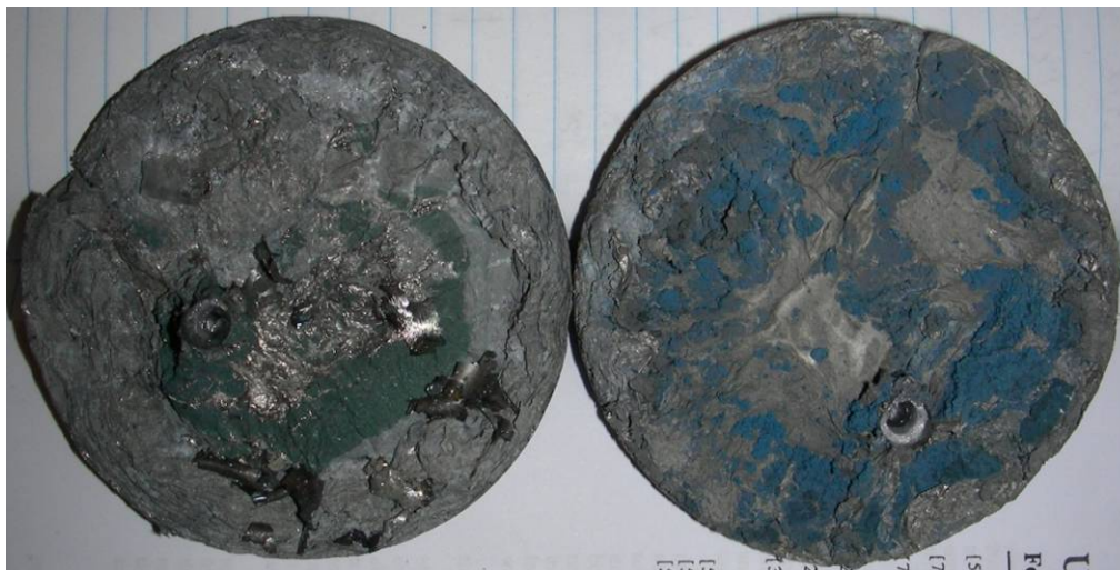
Figure 131. Using quartz tubes as immersion thermocouple protection tubes, and alumina crucibles, CMSX-4 melt slag showed oxidation features.
