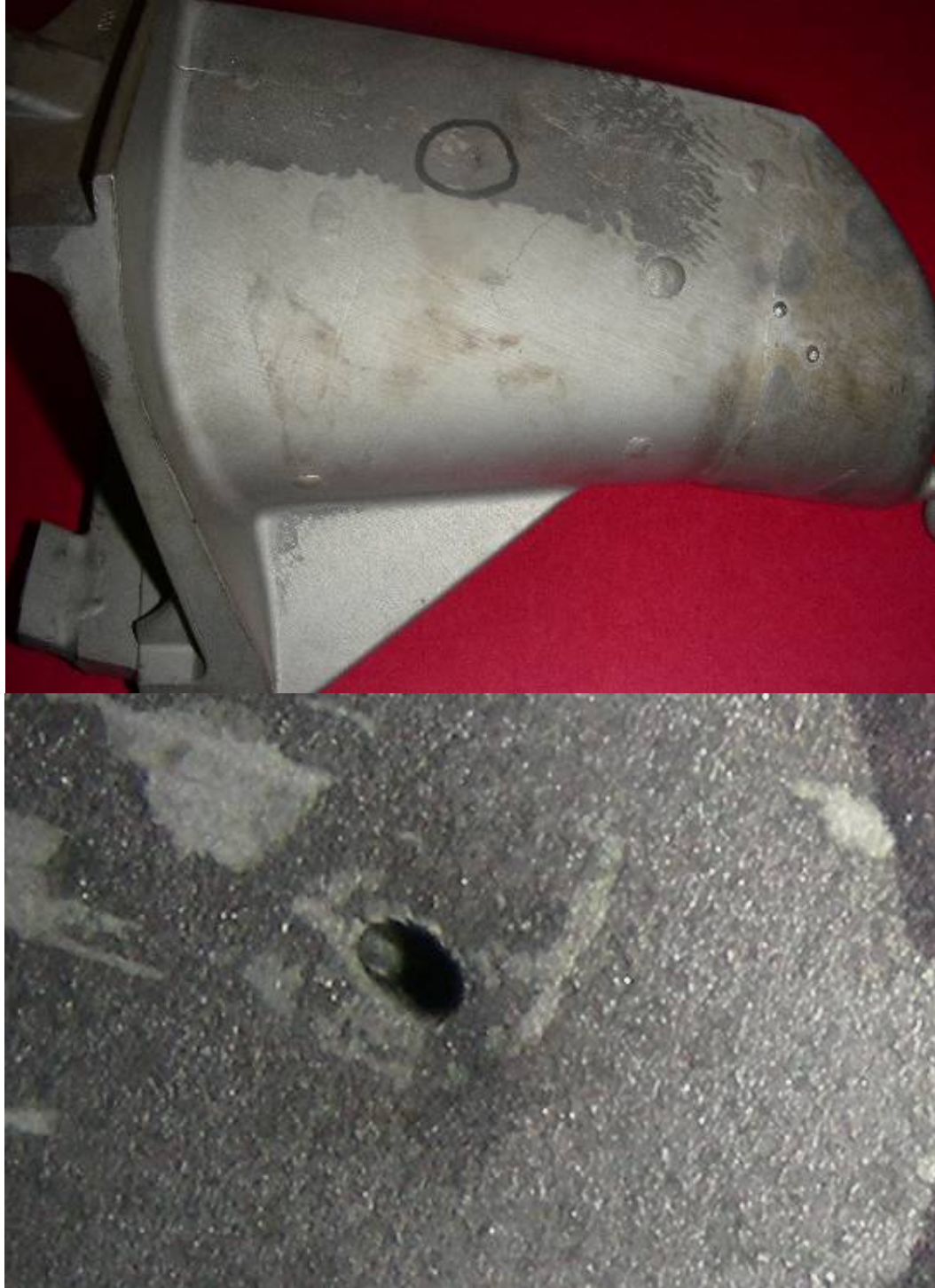
Figure 25. CMSX-4 SX casting with metal mold reaction and gas hole defect.
