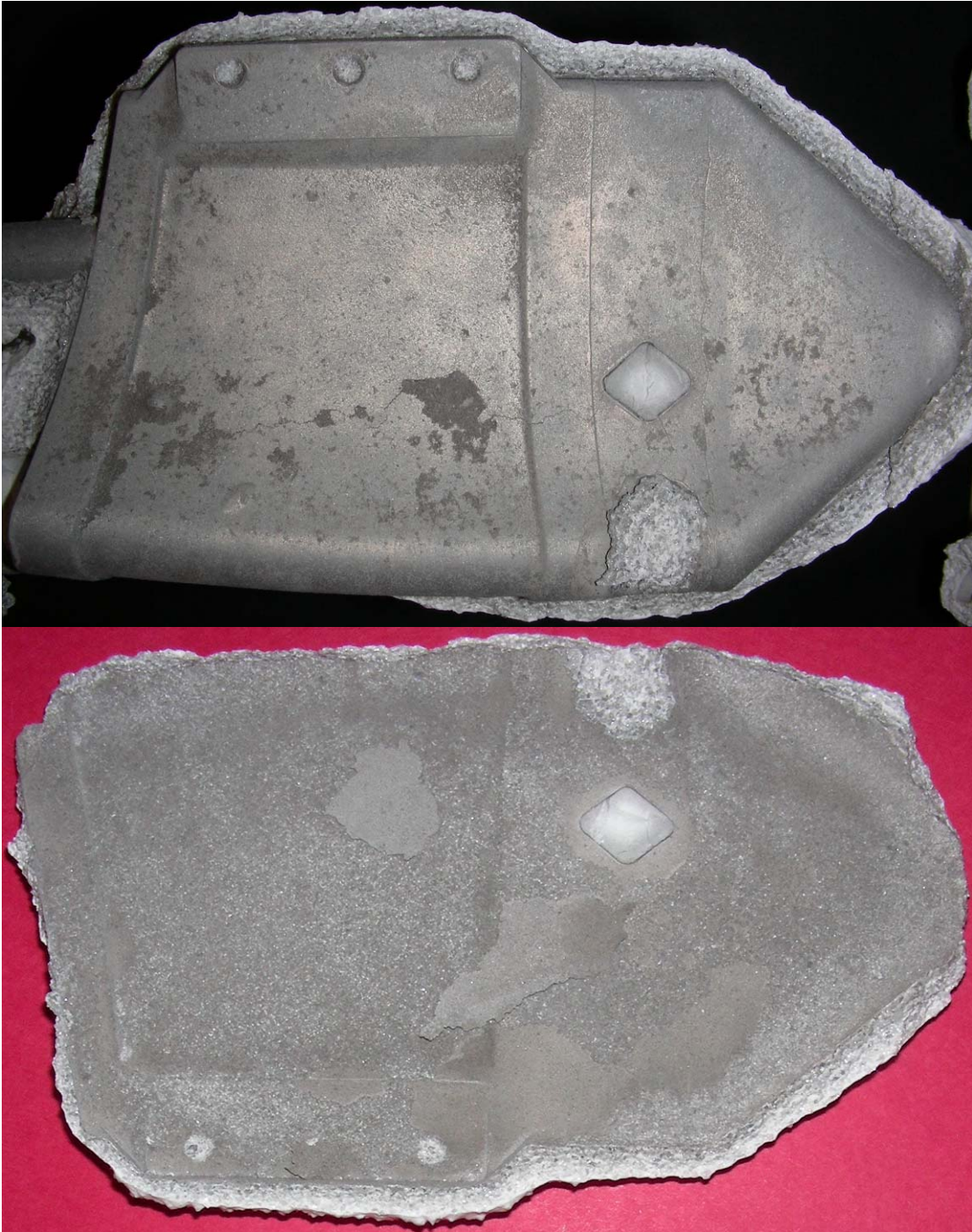
Figure27. CMSX-4 SX casting with metal mold reaction and hot tears defect
