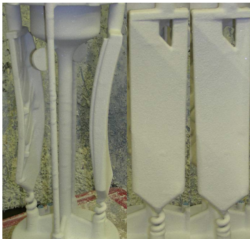
Figure 41. Wax pattern assembly after Y aerosol spray coating, normal zircon facecoating and stuccoing
