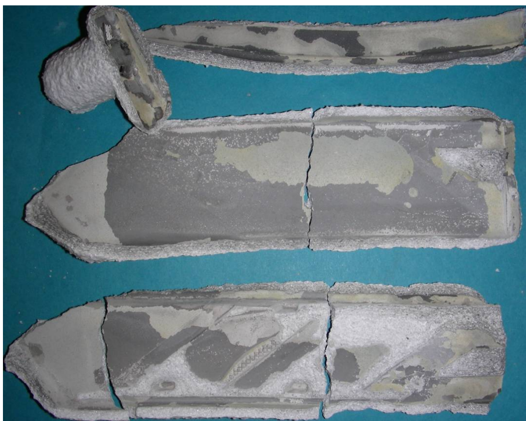
Figure 45. Visual appearance of CMSX-4 casting trial using shell mold with yttria aerosol spray coating and yttria binder washing and soaking.
