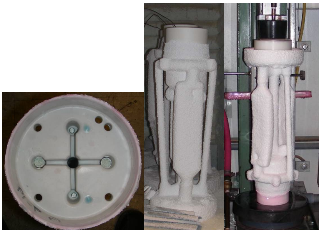
Figure 43. a) Bottom filtration b) Shell mold after burnout/firing c) Washing shell mold after dye penetration inspection
