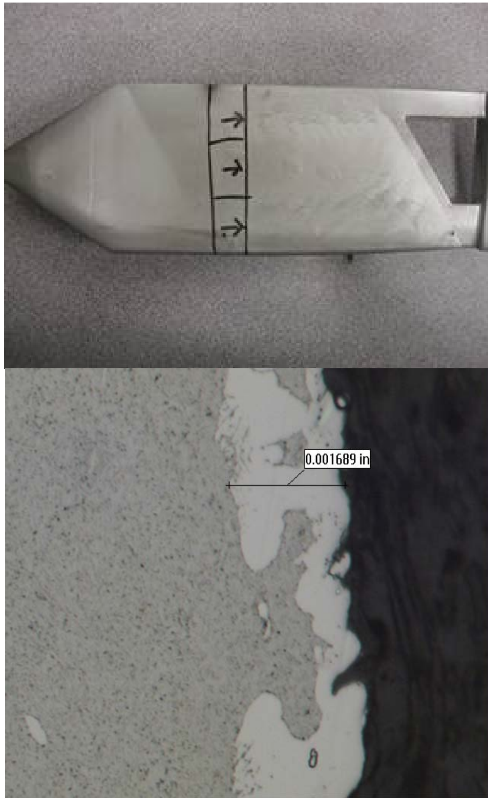
Figure 22.b) A typical metal mold reaction layer on the CMSX-4 platform casting
