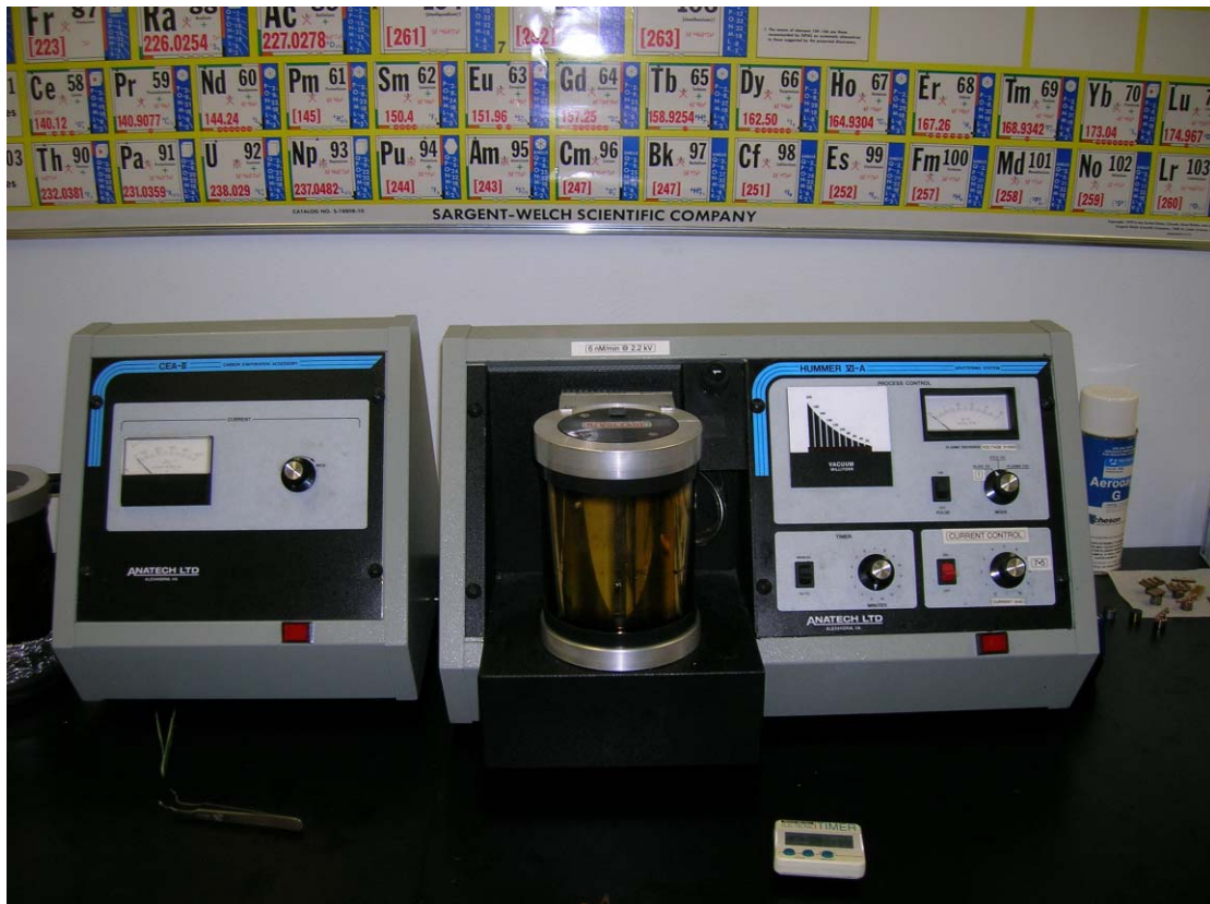
Figure 35. Hummer VI-A Sputtering System (Gold coating)
