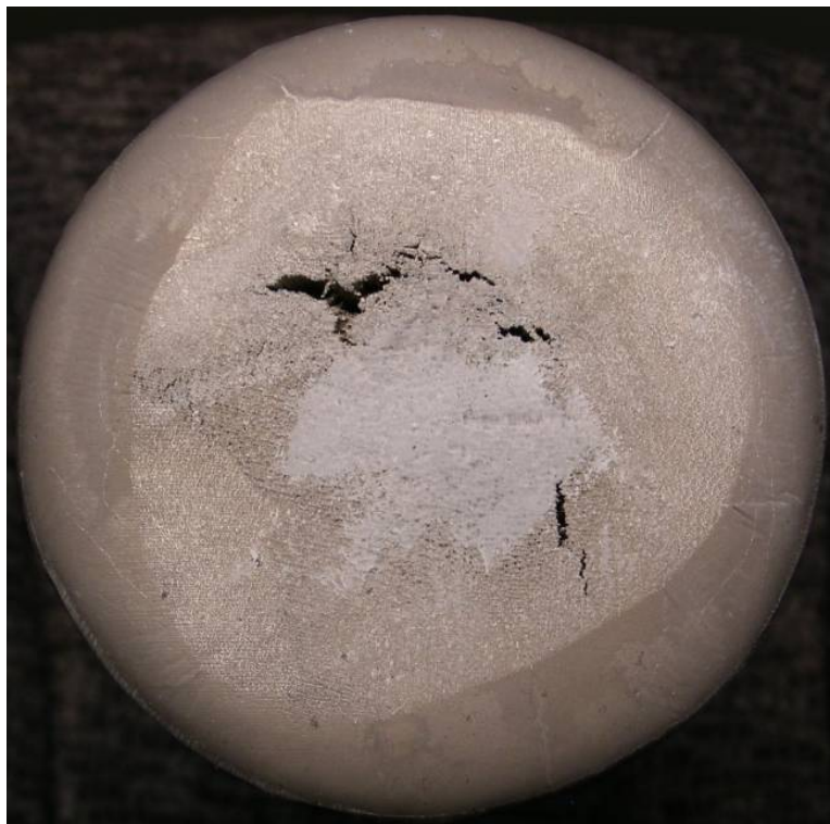
Figure 47. a) Visual appearance of top surface of pouring basin of CMSX-4 casting trial showed some dross.
