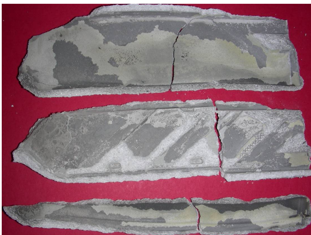
Figure 46. Visual appearance of CMSX-4 casting trial using shell mold with yttria aerosol spray coating but without yttria binder washing and soaking
