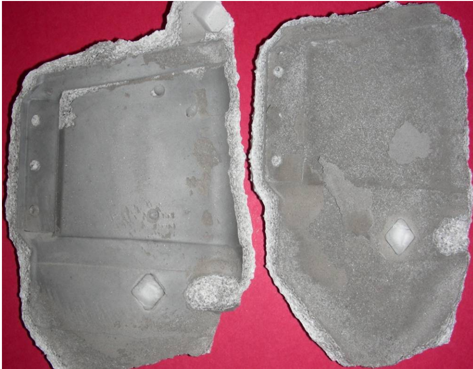
Figure 32. C) Shell molds of CMSX-4 SX castings: Left one (Sample 8) from part with secondary grain defect, Right one (Sample 7) from part with hot tear defect
