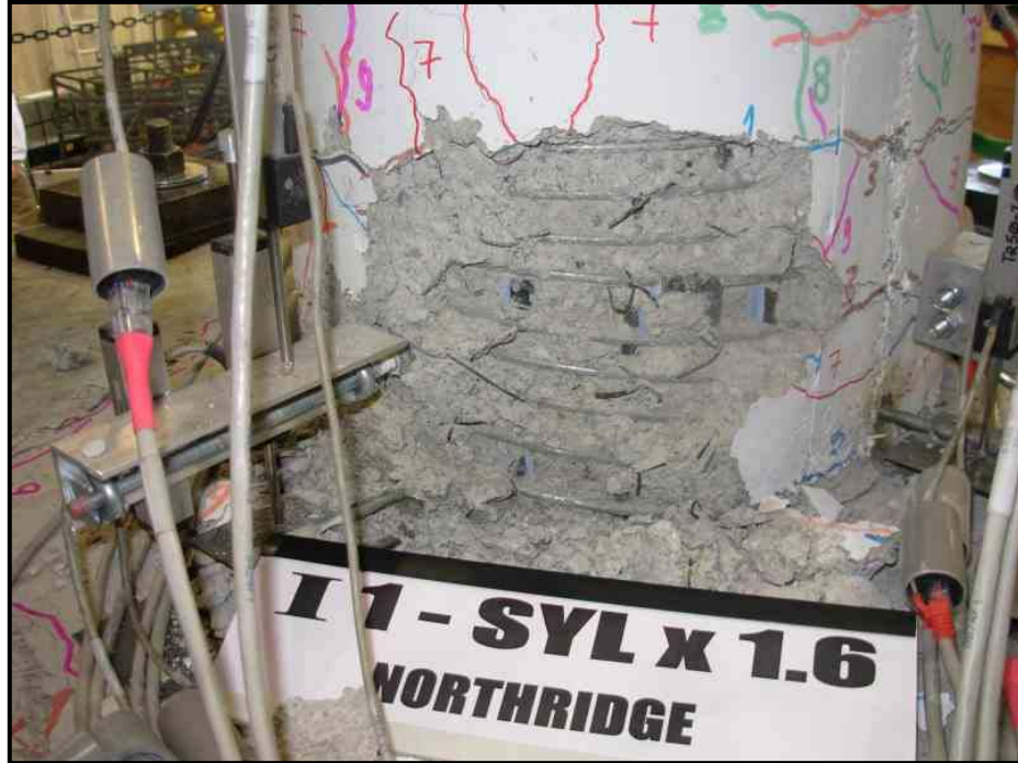
Figure 5-32 Spiral and Longitudinal Bars Visible, Specimen I1
