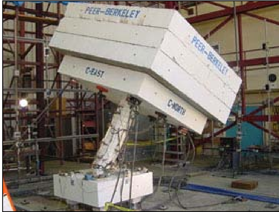
Figure 3-19 Shake Table Testing of Single Cantilever-type Column (Mahin et al. , 2004)
