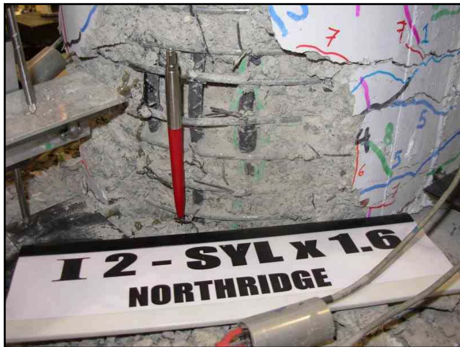
Figure 5-33 Spiral and Longitudinal Bars Visible, Specimen I2
