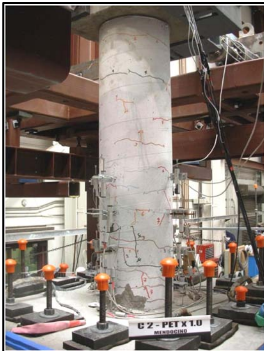
Figure 4-29 First Concrete Spalling Specimens C2 (PETx1.0)
