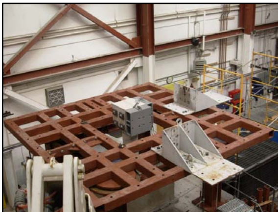
e) Connecting Links on Platform
