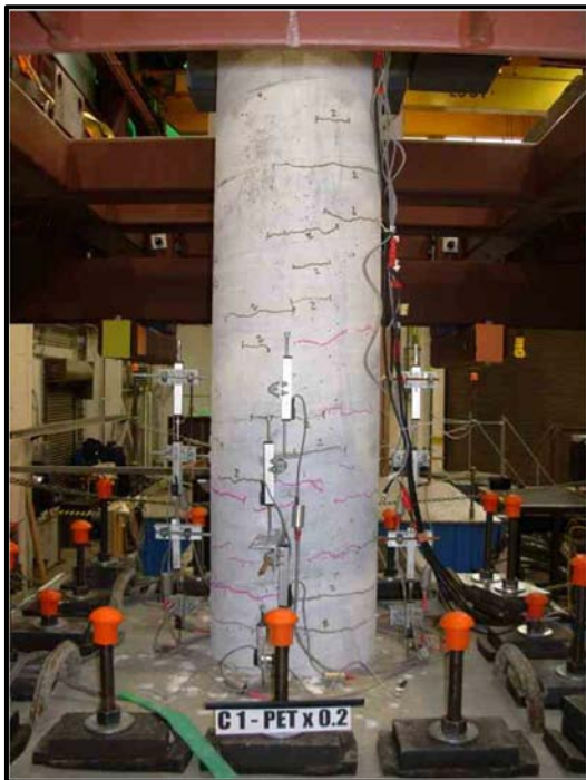
Figure 4-27 Cracks at First Bar Yielding, Specimens C1 and C2 (PETx0.2)
