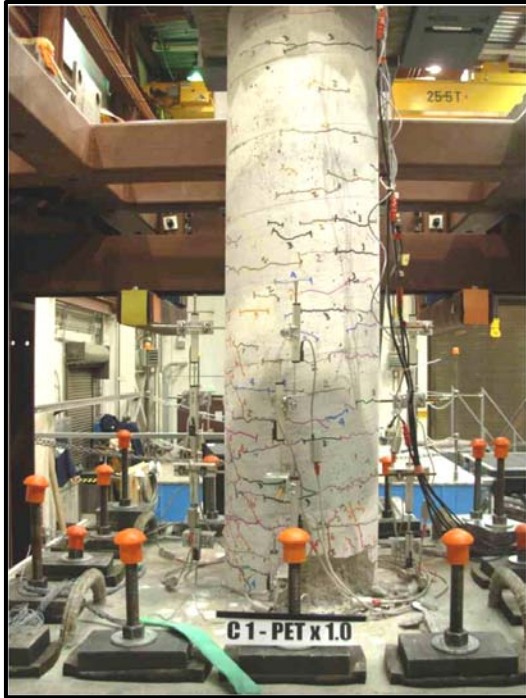
Figure 4-28 First Concrete Spalling Specimens C1 (PETx1.0)
