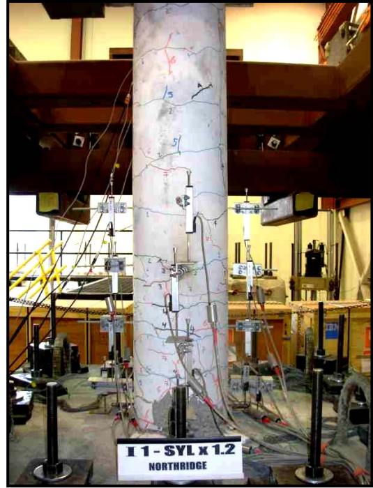
Figure 5-30 Specimen I1, Increasing of Cracks and Spalling (SYLx1.2)
