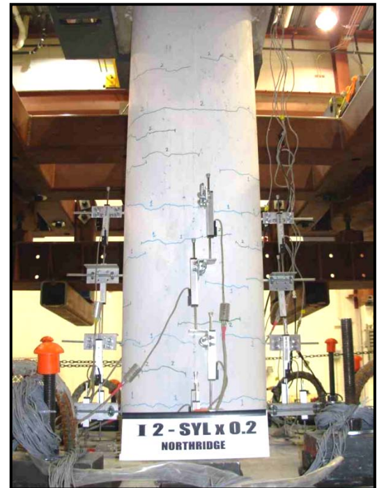
Figure 5-27 Cracks at First Longitudinal Bar Yielding, Specimens I1 and I2 (SYLx0.2)
