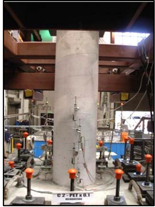
Figure 4-26 Hairline Horizontal Cracks, Specimens C1 and C2 (PETx0.1)
