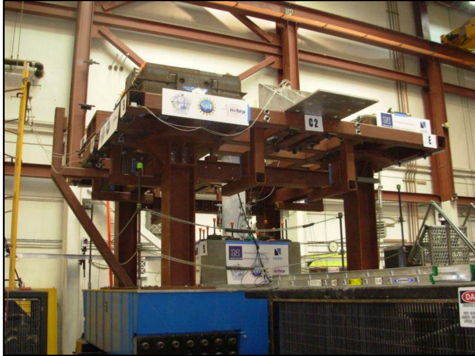
Figure 3-32 Bidirectional Mass Rig and Specimen(Before Testing)
