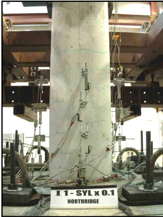
Figure 5-26 Hairline Horizontal Cracks, Specimens I1 and I2 (SYLx0.1)
