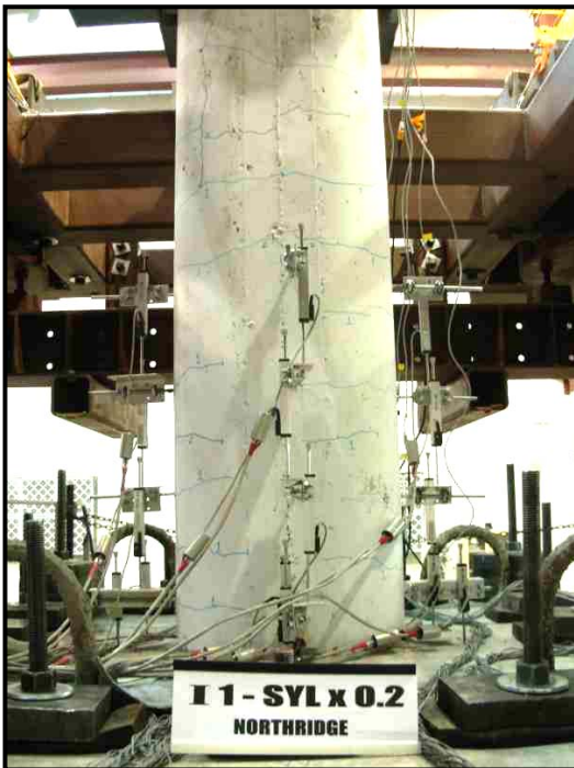
Figure 5-27 Cracks at First Longitudinal Bar Yielding, Specimens I1 and I2 (SYLx0.2)
