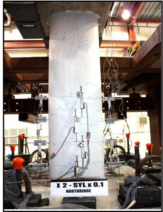
Figure 5-26 Hairline Horizontal Cracks, Specimens I1 and I2 (SYLx0.1)
