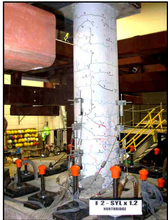
Figure 5-31 Specimen I2, Increasing of Cracks and Spalling (SYLx1.2)
