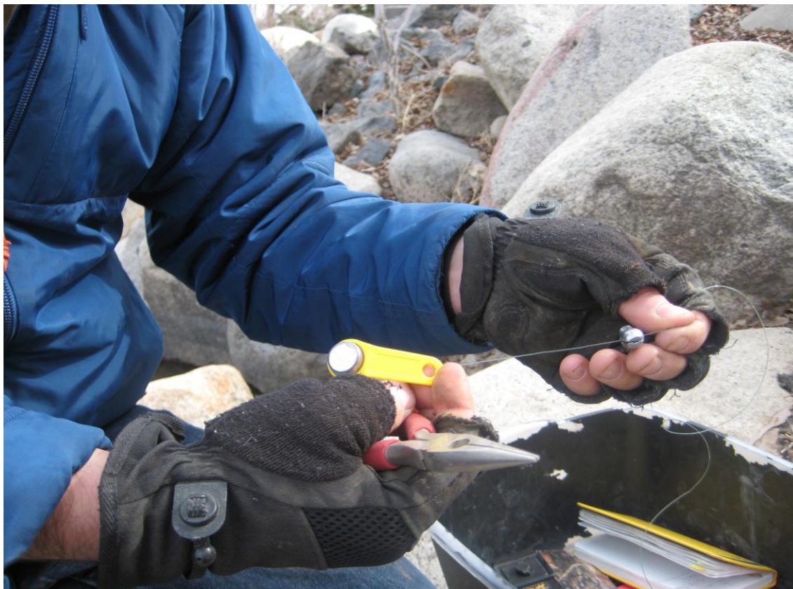
Figure 3.3 Weights tied on thermistors for stability before placing in river.
