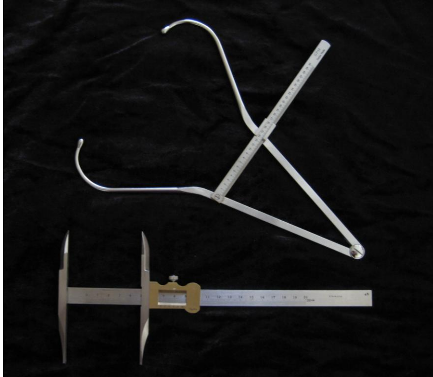
Fig. 3. Spreading calipers (above) and sliding calipers (below) used in taking cranial measurements.
