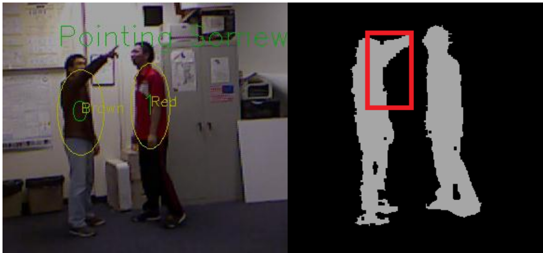
Figure 12. A person's pointing gesture (left); detected foreground objects (right).
