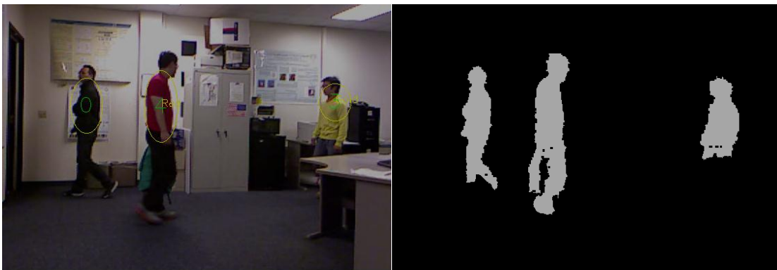
Figure 7. Original image (left); detected foreground (right)
