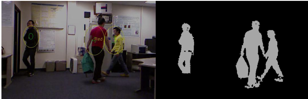
Figure 8. Original image (left); detected foreground (right)
