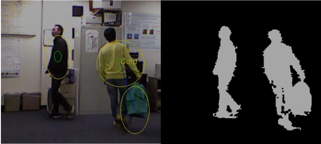
Figure 10. Original image, a person carrying a bag (left); detected foreground (right)
