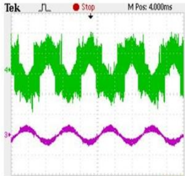
Fig. 4.65 Switched inductor Z-source matrix converter. Top: Output phase voltage bottom: phase output current.
