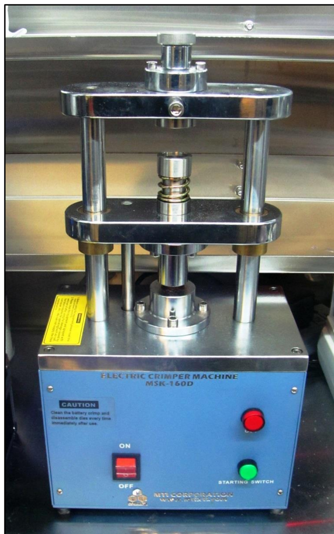
Fig. 13: MTI electric crimper housed inside the glove box. Following assembly by hand, coin cells were crimped to seal contents.
