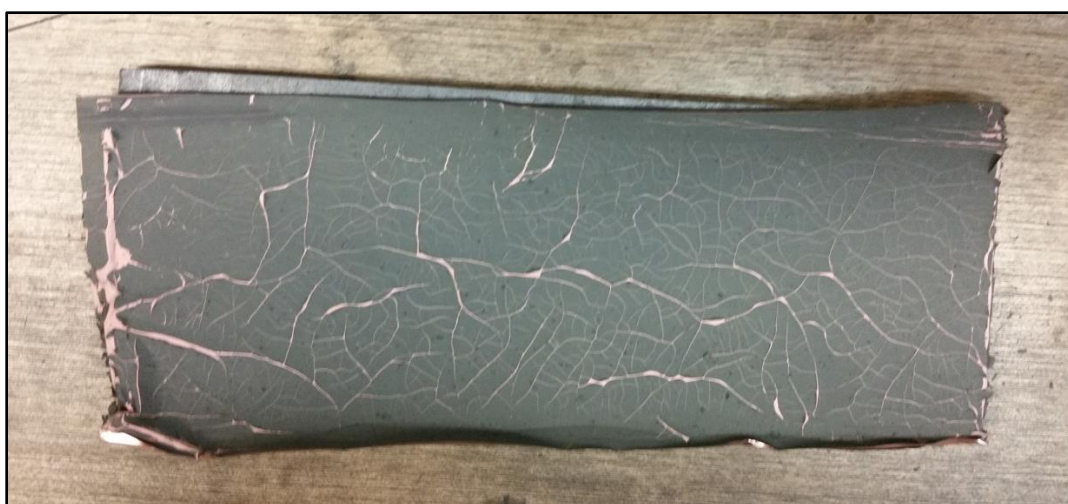
Fig. 3: A slurry-coated foil following the high-temperature heat treatment step in the tube furnace. It is speculated that the ramp-up heating rate programmed for the furnace was too fast.
