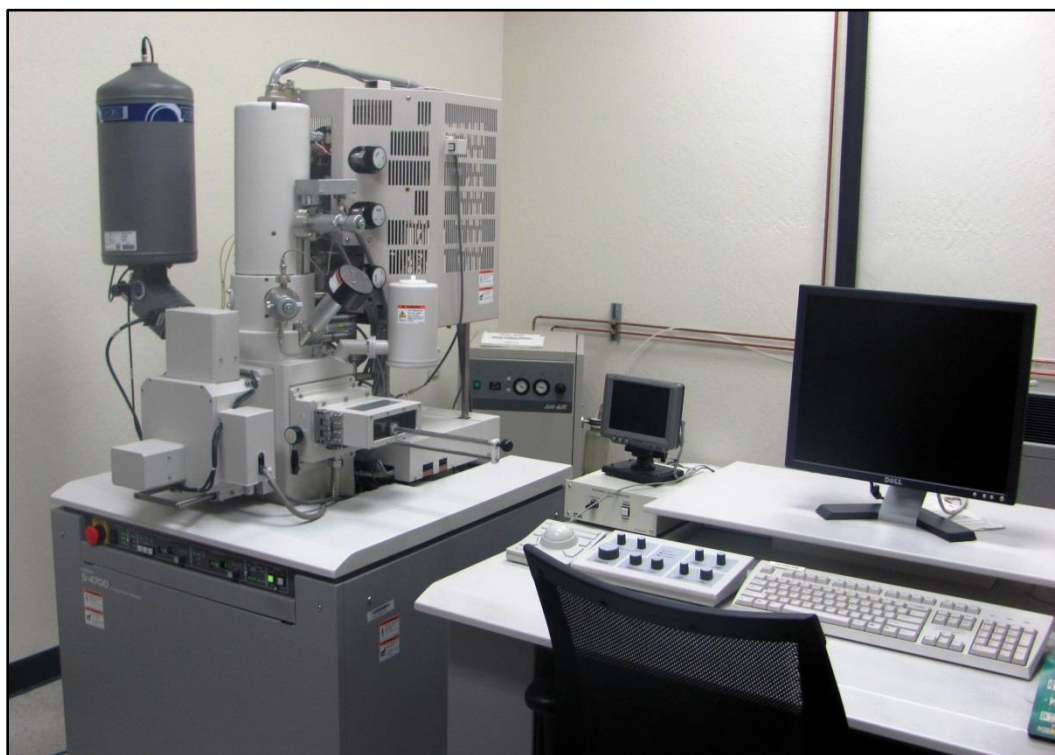
Fig. 15: Hitachi S-4800 scanning electron microscope (SEM) and attached Oxford energy-dispersive X-ray spectroscopy (EDS) system used for surface characterization of the samples.
