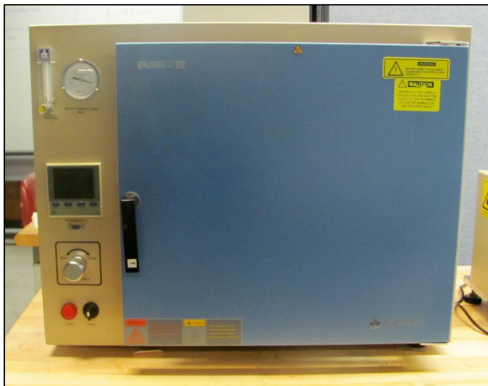
Fig. 7: MTI vacuum oven used for low temperature heat treatment of the coated foils. Foils were heated at 120°C for 12 hours.
