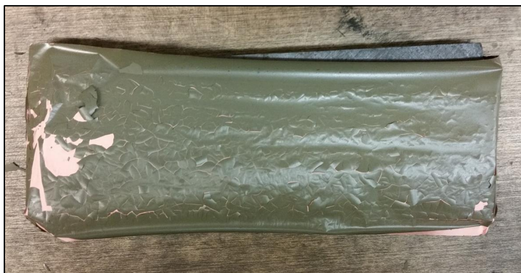
Fig. 2: A dried, slurry-coated foil with severe cracking and poor adhesion visible on the surface. During mixing, the binder was not fully integrated into the slurry.
