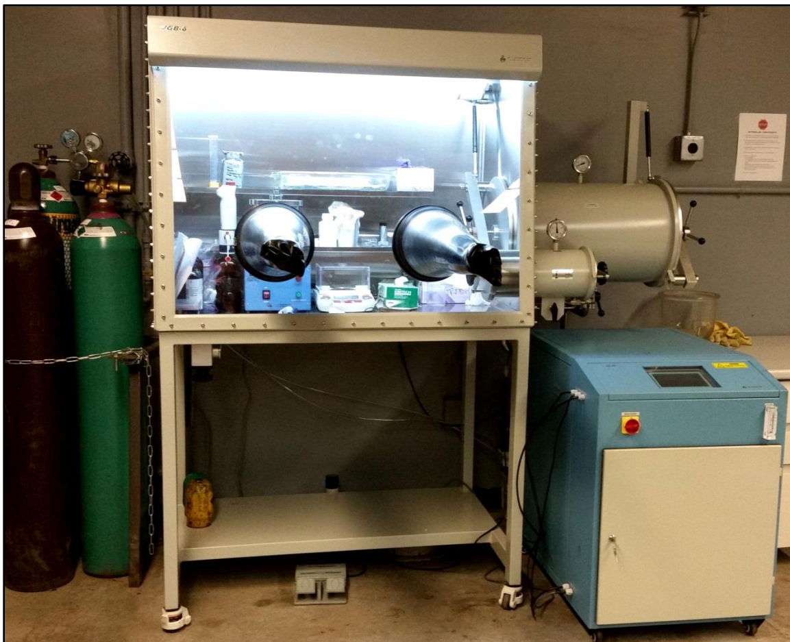
Fig. 12: Glove box used for coin cell assembly. Glove box conditions were maintained with water and oxygen content less than 1.0 ppm.
