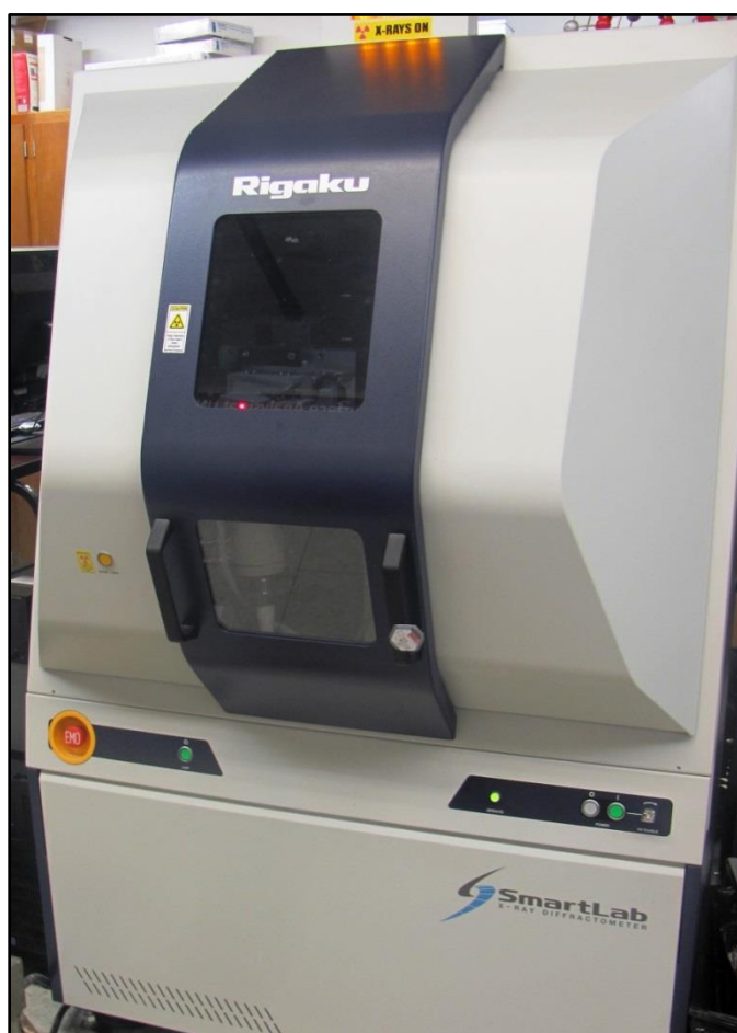
Fig. 18: Rigaku SmartLab X-ray diffractometer (XRD) used to characterize the anode samples. All patterns were collected over the range of 2\theta = 20^\circ to 100^\circ with a step size of 0.07^\circ and at a scan rate of 0.5^\circ\text{min}^{-1} .
