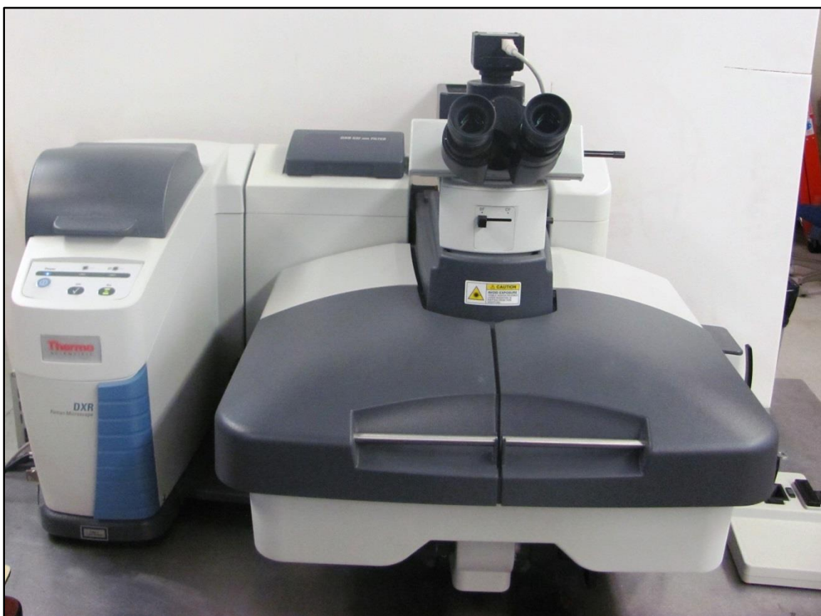
Fig. 17: Thermo Scientific DXR Raman Microscope used for characterization of the anode disc surfaces. Data were obtained at 10x magnification and a spot size of 50 \mu\text{m} .
