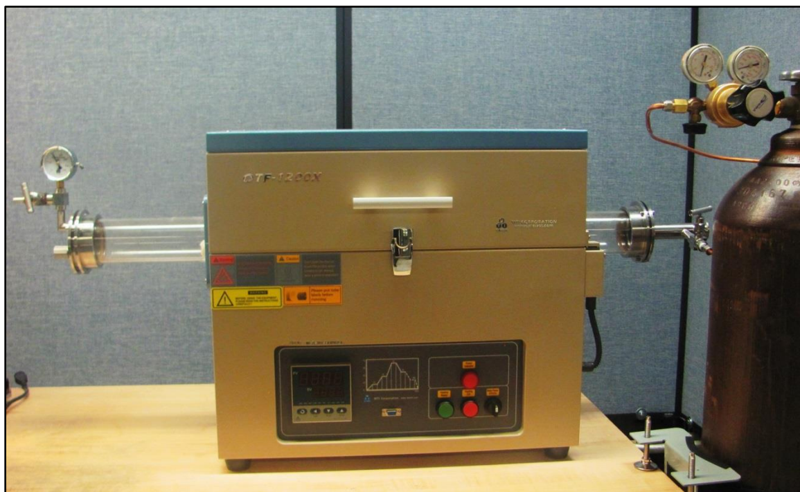
Fig. 9: MTI tube furnace used for high temperature heat treatment of the coated foils. Foils were annealed under argon for 700°C for 15 minutes. A graphite stage was made to keep the foils flat while inside the tube.
