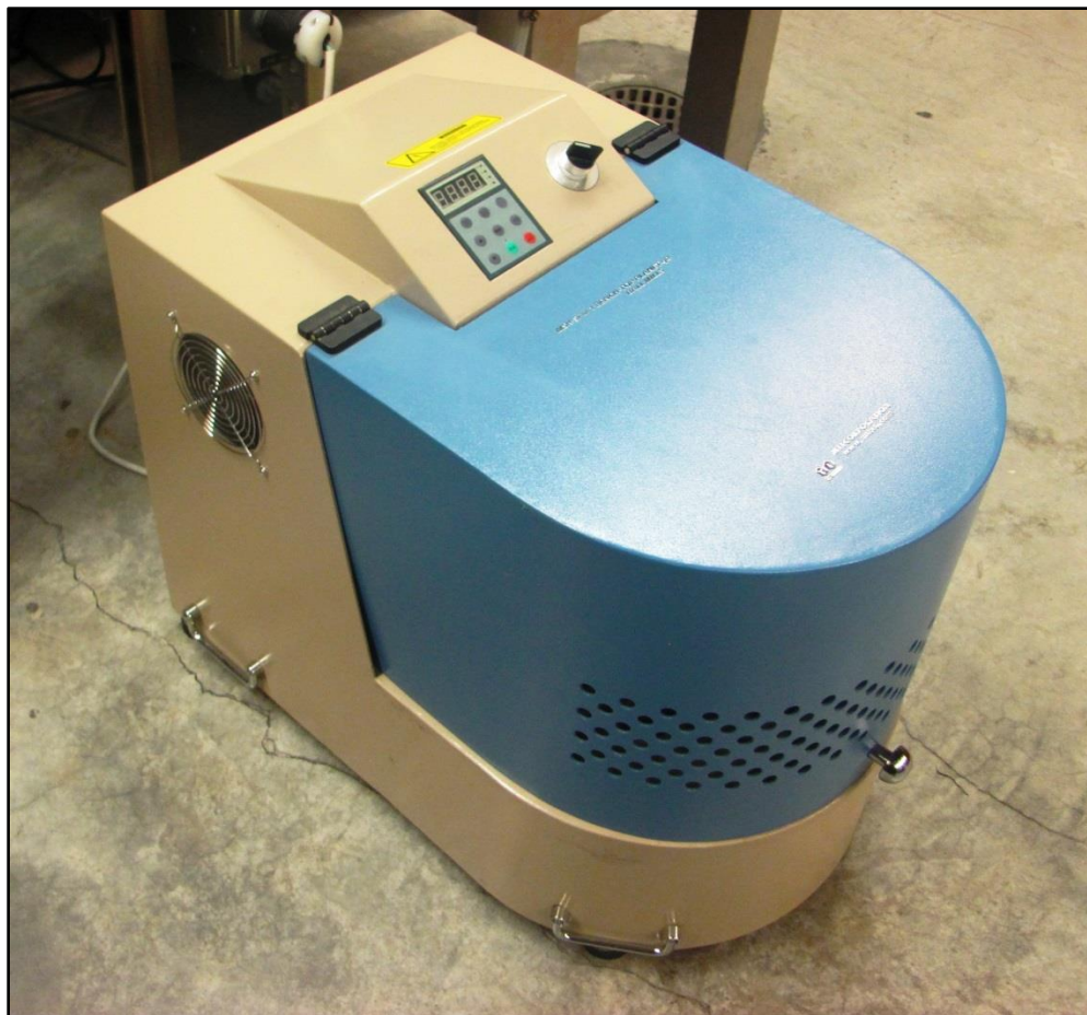
Fig. 5: MTI Planetary ball mill used to reduce the particle size of dry material. The ball mill was operated for 30 minutes.
