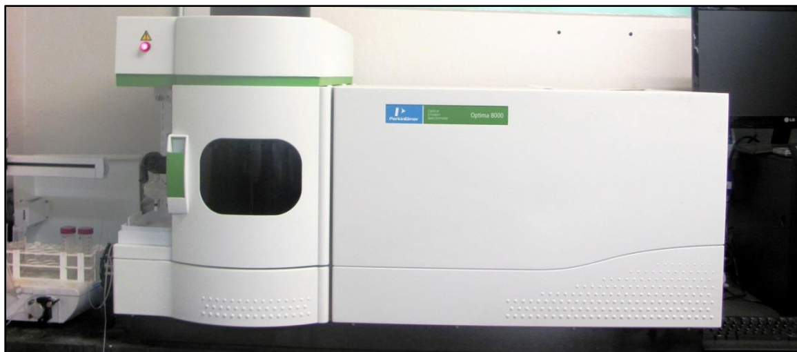
Fig. 16: PerkinElmer inductively couples plasma optical emission spectrometer (ICP-OES) 8000 used to assess the copper content of anode materials after heat treatment.
