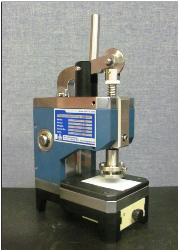
Fig. 11: MTI disc punch for preparing separator discs from sheets of Celgard tri-layer PP/PE/PP membrane. Discs of 18 mm diameter were used.
