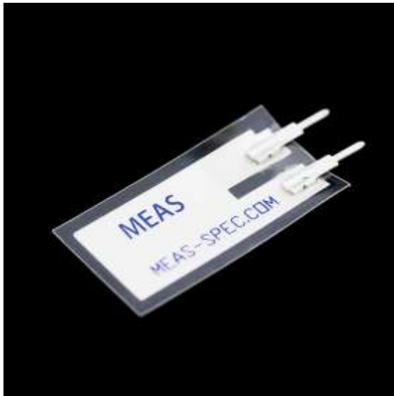
Figure 6.21: Piezoelectric film used for experiments and its dimensions (adopted from Sparfun Electronics)
