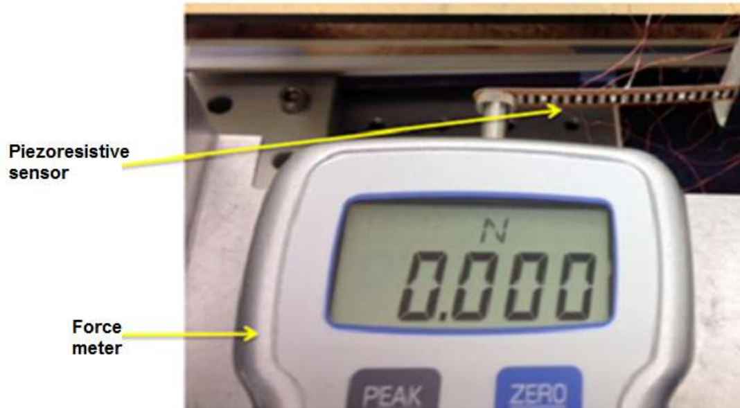
Figure 6.7: Actual experimental setup for the piezoresistive sensor
