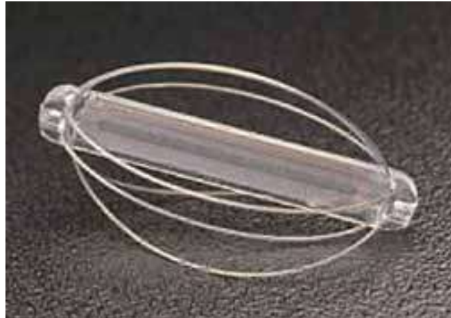
Figure 3.2: Endovascular wireless pressure sensor (adopted from [38], Silveira P.G., Miller C.W.T.. et al)
