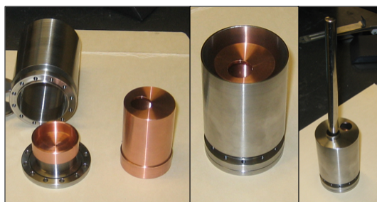
Figure 4.9: A photograph of the sample chamber parts: copper pot, copper stage, steel pot and steel tubes.
