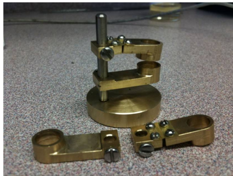
Figure 4.11: Photo of brass transducer stage arms and platform. Two sets of arms were built, as shown. Only one set was used during a particular experiment.
