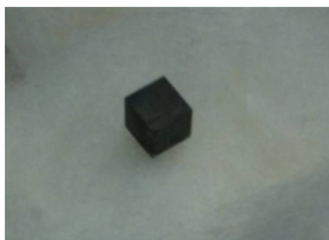
Figure 4.6: A photograph of a completed parallelepiped Gd sample.
