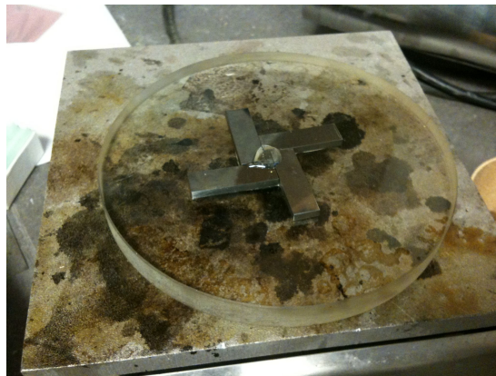
Figure 4.5: Photograph of the polishing platform with right angle blocks.
