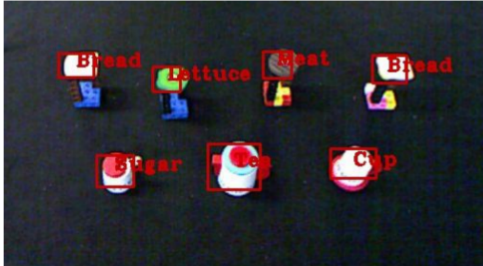
FIGURE 4.2: An example detection and recognition by the vision part using the Kinect camera on the PR2.
