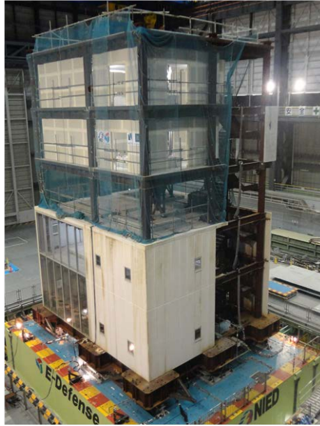
Figure 2-1: The 5-story steel moment frame specimen
