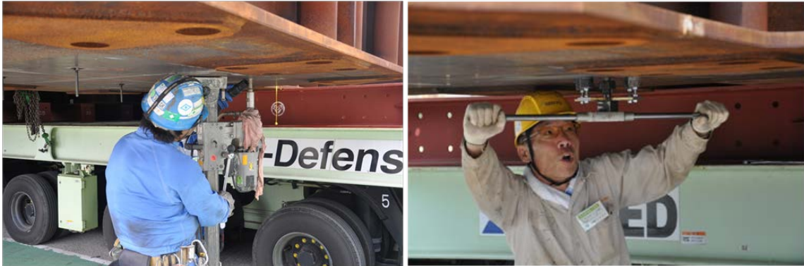
Figure 4-17: Drilling and tapping holes at the bottom of the specimen
