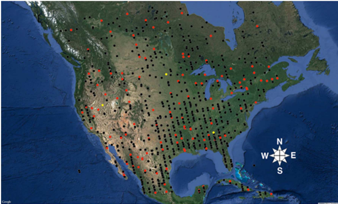
Figure 13. Map of absolute mixing height difference across methods (for TKE, RI, and Stull) from RUC2 (lidar excluded). Red (black) dots indicate differences above (below) 500 m, respectively. The three yellow dots demark case example locations to be examined for the Southeast, Northern Plains, and Western US (east to west), respectively.
