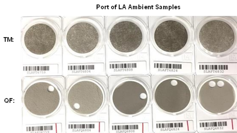
Figure 2-17. Photos of TM and QF filter samples from the Port of LA TIPP site. TM samples are above their QF counterparts. 0.5 cm 2 punches were removed previously from QF filters for carbon analysis.
