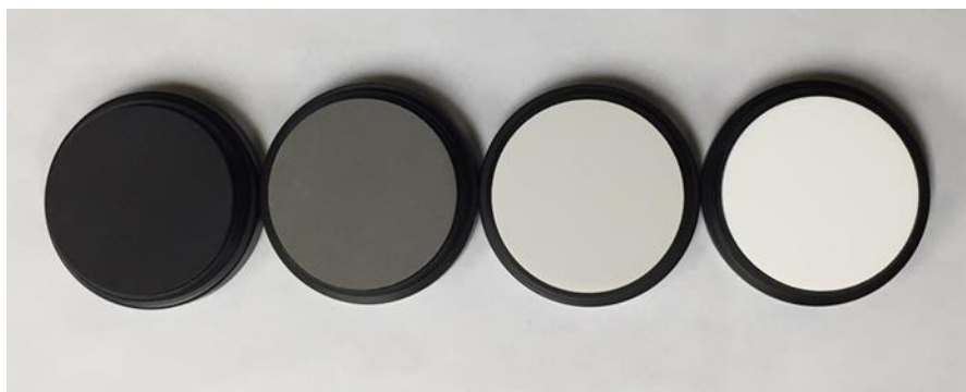
Figure 2-4. Spectralon® reflectance standards. From left: 5%, 20%, 75% and 99% reflectance.
