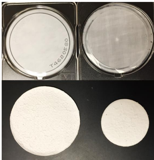
Figure 2-8. Blank filters. Top: Teflon-membrane (TM). Bottom: Quartz-fiber (QF). TM can vary in opacity and QF can vary in surface roughness.
