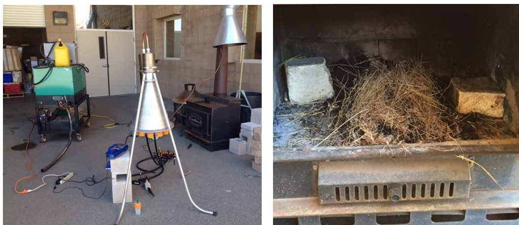
Figure 2-12. Layered source sampling set up. At left, a photo of the manifold set up for use in collecting the layered samples. Also shown in this photo are the diesel generator used for exhaust sampling and the outdoor stove used to burn cheat grass. At right, a photo of cheat grass in stove before being burned.
