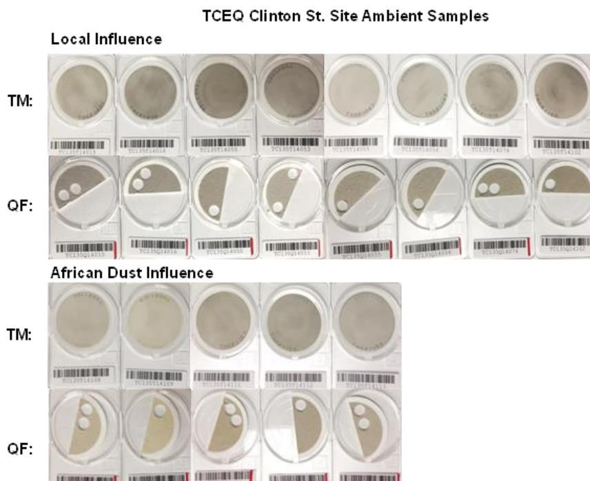
Figure 2-15. Photos of TM and QF filter samples from the TCEQ Clinton St. Site. The top two rows are samples from local influence and the bottom two rows are samples from a time of African dust transport. TM samples are above their QF counterparts. 0.5 cm 2 punches were removed previously from QF filters for carbon analysis.
