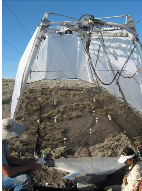
Figure 6: Walnut Gulch rainfall simulator operating at Dry-X.
