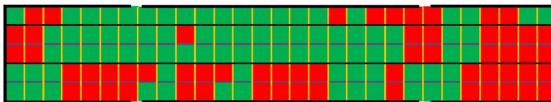
b) Ground Motion 9: Measured PFA= 2.35g, 41.4% Failed Area
