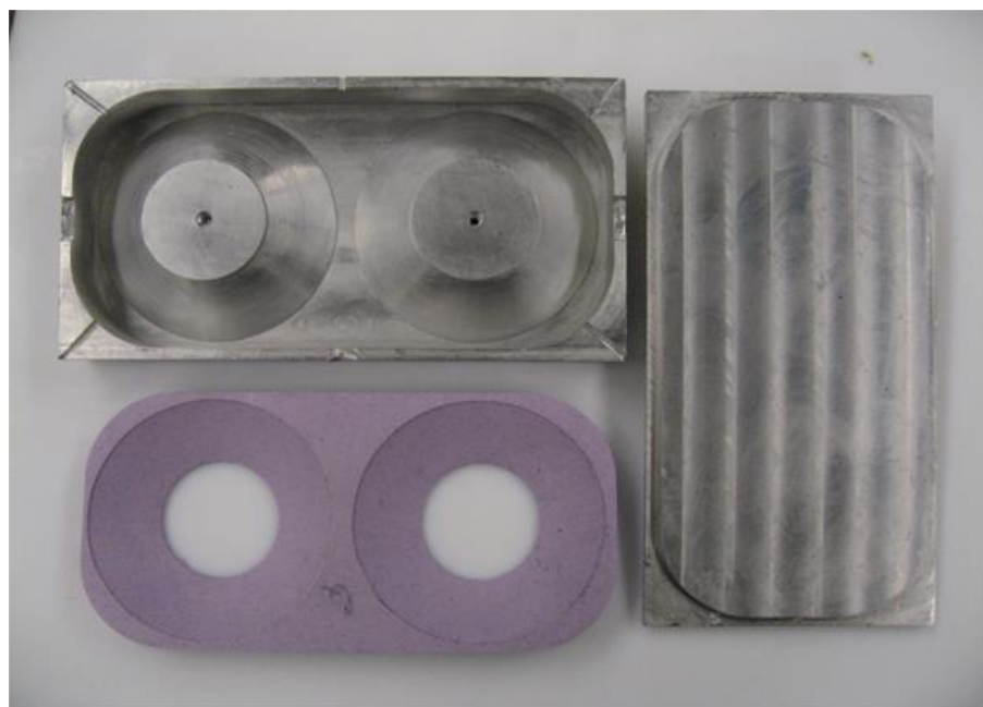
Figure A.3. The fabricated rubber support and mold.
