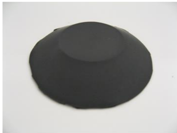
Figure A.2. Silicone-RTV MRE with 70% wt. iron.
