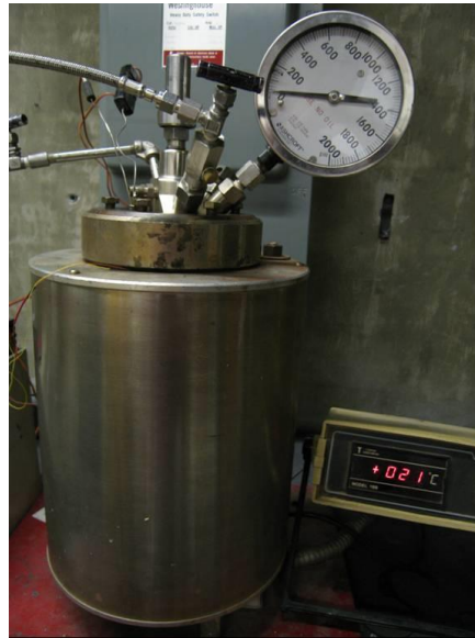
Figure 3.5. High pressure reactor for MRE ageing.
