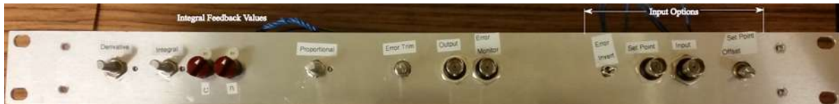
Figure C.4: PID front panel with input, output and control options.
