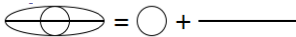
Figure 8: A schematic representation of decomposing an elliptical generic tensor into a ball component and a stick component
