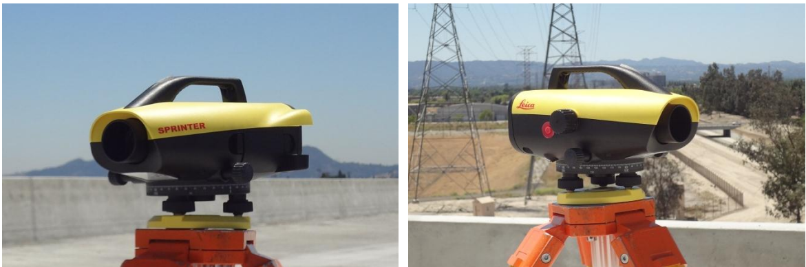
Figure 3-3 Digital level used in field measurements (Sprinter 250M)
