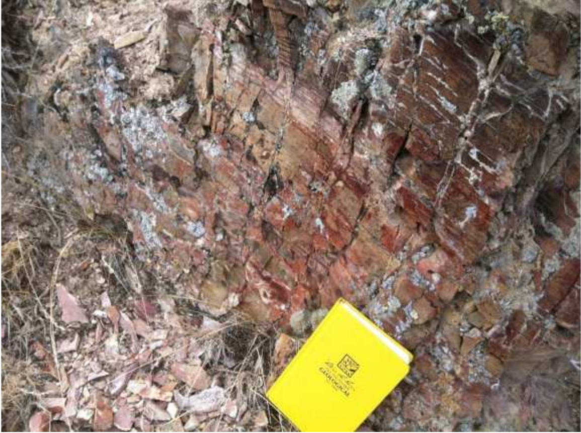
Figure 10. Photo of recessively weathering, very fine-grained, pink silty quartz arenite that is characteristic of Ocl S 2 . Outcrops of this unit are rare at Iron Point.
