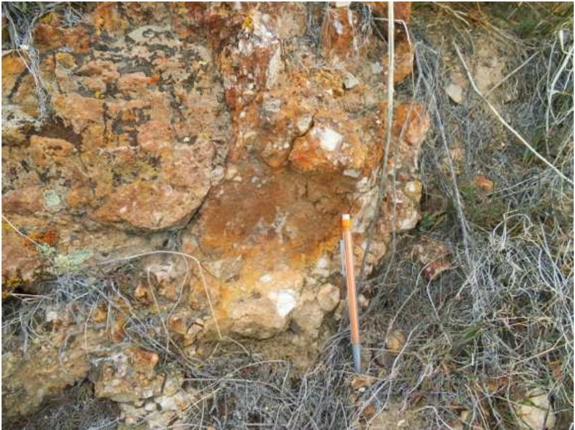
Figure 22. Breccia within the newly identified unit Oe. Matrix is fine- to very fine-grained sand and angular white clasts are quartzite.
