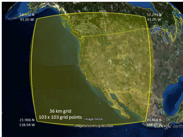
Figure 7: The above image displays the horizontal area of the 36 km resolution inner domain.
