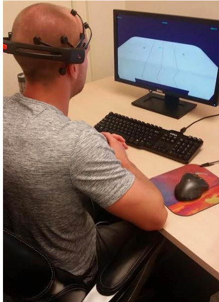
Figure 5.15: Player using the Emotiv Epoc’s BCI controls to interact with the 3D Air Hockey game.
