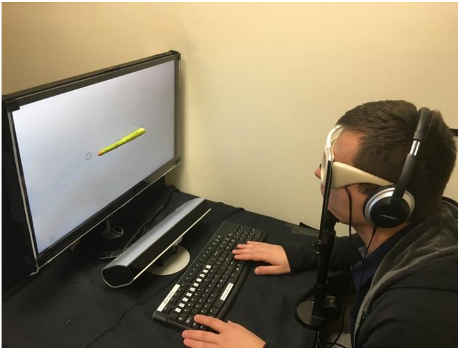
Figure 1. Display Setups Experiment 1. The LCD monitor was positioned at 57 cm from the observer. Participants wore noise-cancelling headphones that played white noise. Viewing time was controlled using LCD glasses in both the picture and real object conditions. A chin rest was used to control viewing distance, and to reduce head movements.
