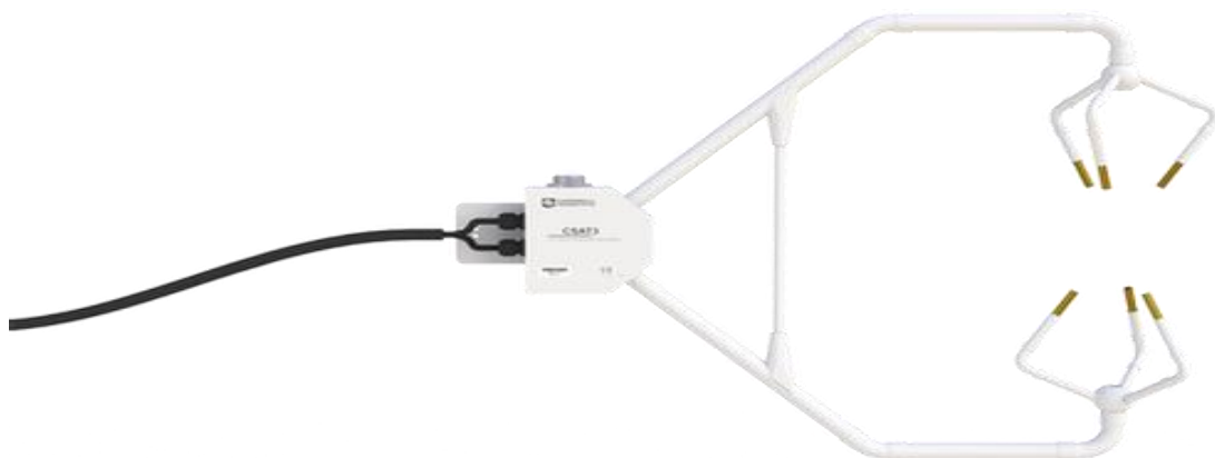
Figure 2.3. Photograph of the CSAT3 sonic anemometer. [Image Reference: https://www.campbellsci.com/irgason ].
