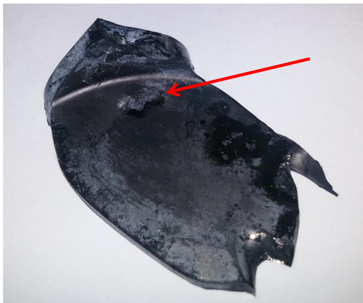
Figure 3.3: A shard of a vitreous carbon crucible that failed during a 20 hour exposure to molten \text{LiCl-2wt\%Li}_2\text{O-1wt\%Li} at 650^\circ\text{C} . Localized corrosion was observed (indicated by the red arrow) suggesting that the material was chemically attacked by the molten solution.
