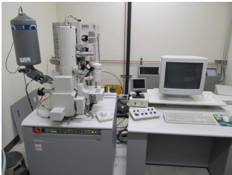
Figure 2.6: Hitachi S-4700 field emission scanning electron microscope, equipped with an energy dispersive spectrometer.
