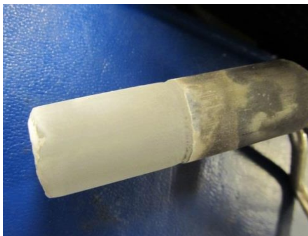
Figure 3.1: A digital image of Al 2 O 3 after 20 hours of exposure to LiCl-2wt%Li 2 O-1wt%Li at 650°C. The recorded corrosion rate exceeded 50 mm/yr indicating the highly reactive nature of Al 2 O 3 with melts containing metallic Li.
