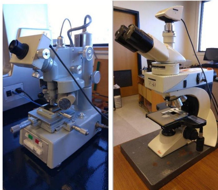
Figure 2.10: The Shimadzu Seisakusho LTD NT-M001 micro-Vickers indenter (left) and the Leica MC170 optical microscope (right) used in this study to evaluate the hardness of samples.
