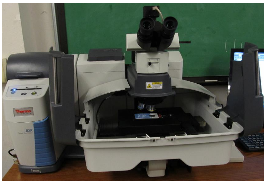
Figure 2.12: Thermo Fischer DXR Raman microscope. The DXR was equipped coupled to a fiber optic probe (not shown) to facilitate Raman spectroscopic analysis of samples in the experimental glove box.
