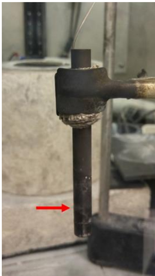
Figure 2.5: The Li-Bi reference electrode used in Chapter 4 of this study. The thin walled graphite tube that contained the molten alloy was held via ceramic insulation outside of the melt and electrical contact to the potentiostat was made through a Ni wire. A red arrow is included indicating the level of the Li-Bi alloy within the reference electrode.
