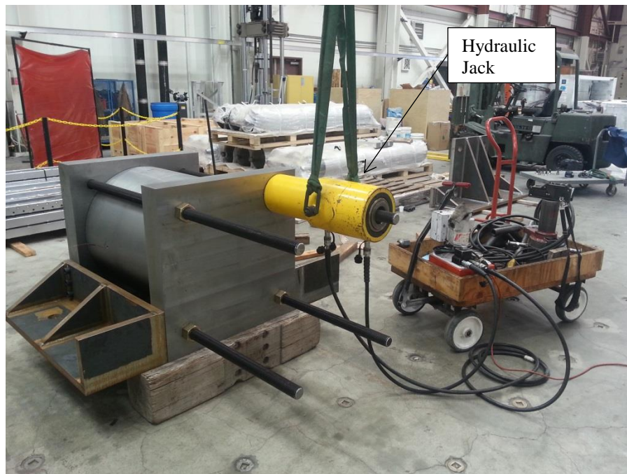
Figure 3.2. Tensioning of the BLS-CMRD with a hydraulic jack.
