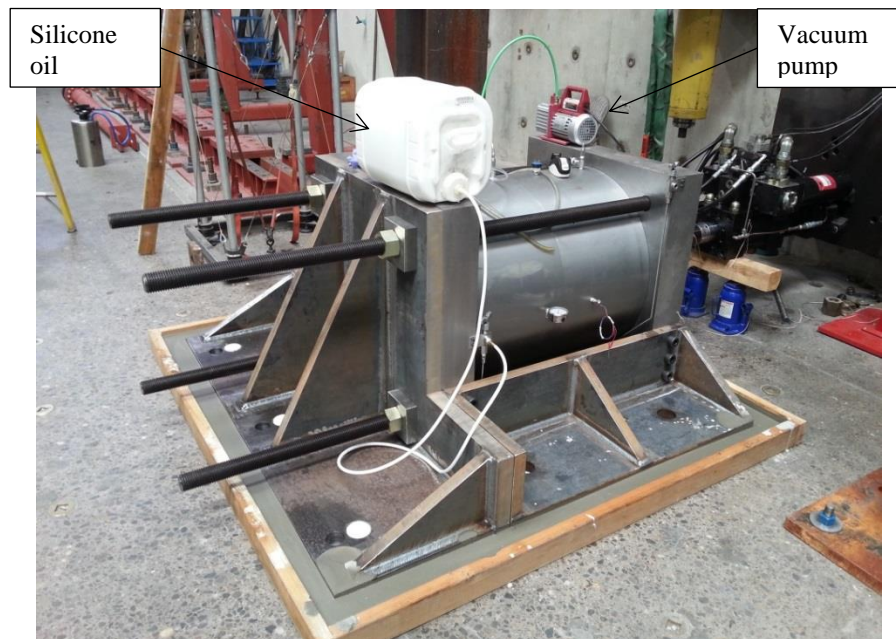
Figure 3.4. Filling the silicone oil into the bottom chamber.
