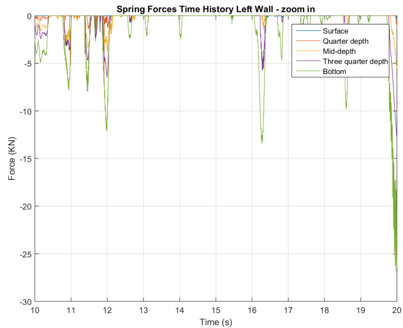
Figure 5-41: Zoom-in of vertical spring forces at five different heights of the left wall of the soil-box, for the model with linear springs (top) and compression only springs (bottom)
