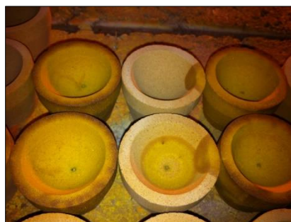
Figure 26. Doré Bead Containing Gold and Silver in Cupels
