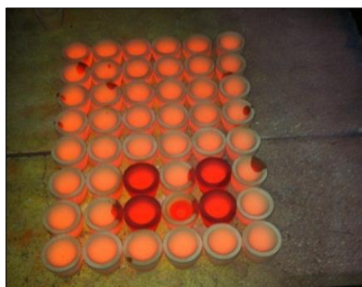
Figure 25. Removed Cupels from the Furnace
