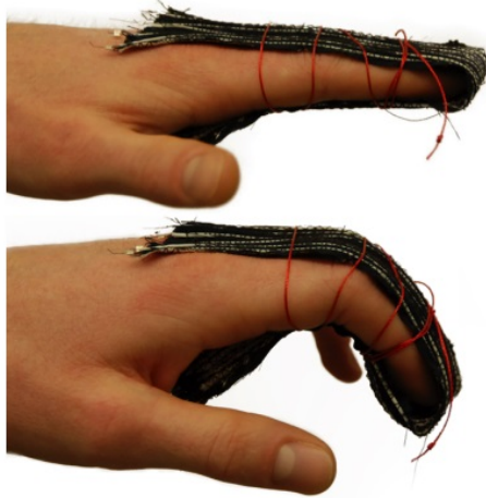
Figure 1.17: Wearable tunable stiffness fabric made from shape memory alloy [13].
