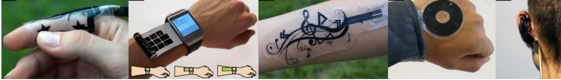
Figure 1.4: ISkin can be worn directly on the skin. Wigel et al. presented (from left to right) FingerStrap, one-handed control of telephone calls; extensions for wearable devices; SkinStickers, input surface for a music player attached; a click wheel on the back of the hand; and a headset control behind the ear [3].
