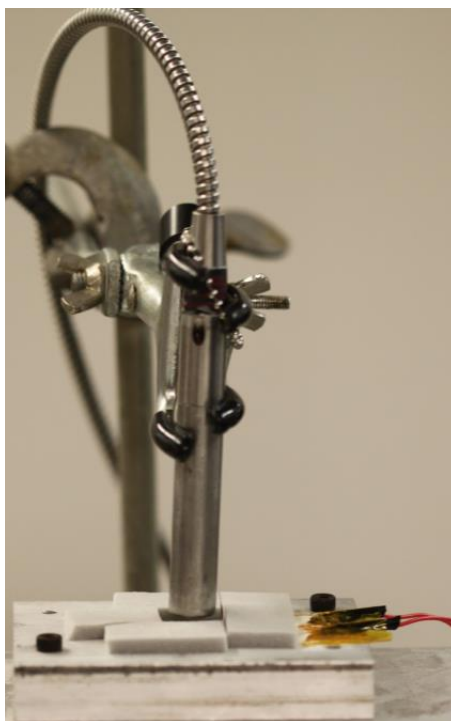
Figure 3.2: Fiber optic probe test setup for the sample characterization tests after removing the foam housing that was used to shield the setup from the ambient air. The focal distance between the fiber optic probe and the sample remained around 4\text{ mm} throughout all of the tests.
