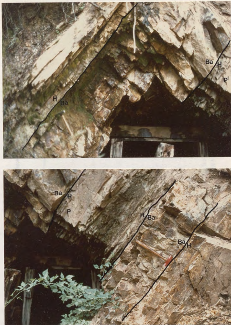
Figure 9 Photographs of bedded barite exposures, Almanor deposit. Barite layers are marked "Ba"; host rocks are marked "H". Point "P" is common to both photographs.
