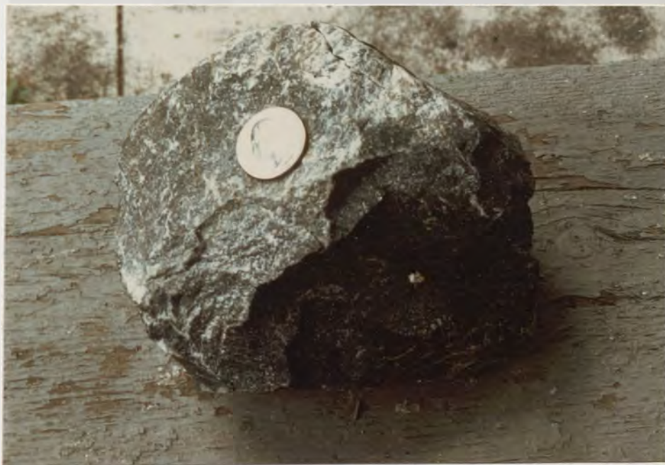
Figure 22 Photographs of barite samples, Glidden deposit. Top: laminated barite and fine grained quartz, light brown and gray laminae are barite, dark brown laminae are iron stained quartz siltstone; bottom: massive barite.
