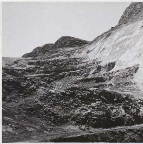
Fig. 2 - Showing "bacon rind" appearance of beds in lower portion of the manganese zone. Massive manganese oxide beds have been stripped off. East end of A pit.
