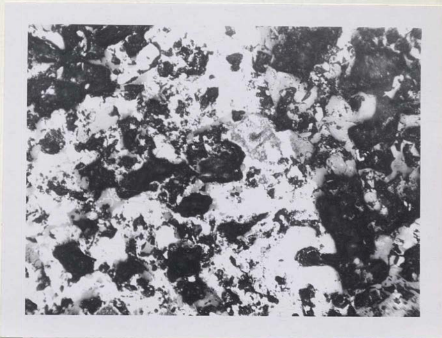
Fig. 6 - Manganese oxides (black) in tuff (white) being replaced by quartz (gray), (X100).
