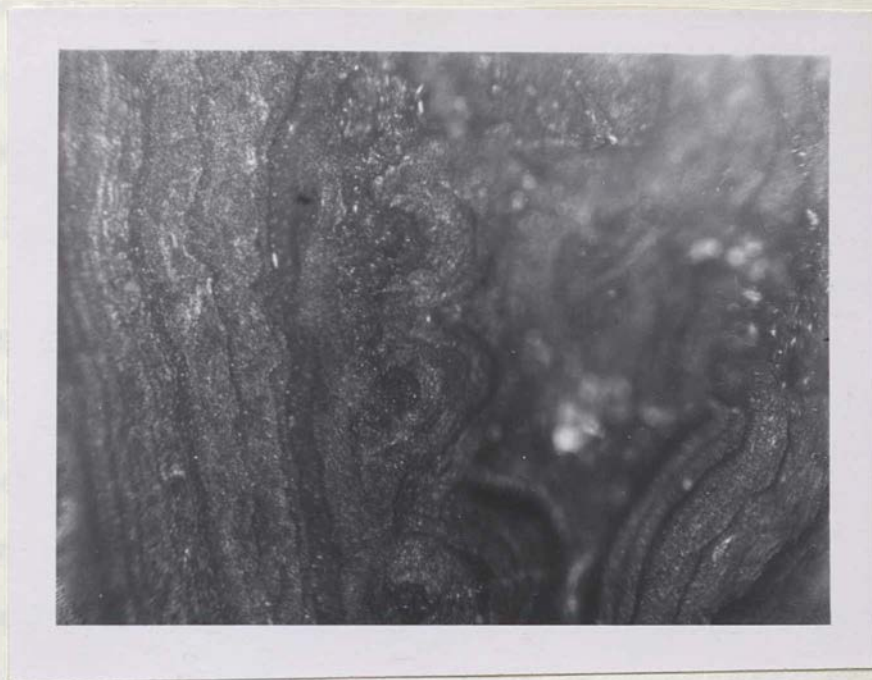
Fig. 8 - Polished section of manganese oxide showing colloform texture, (X100).
