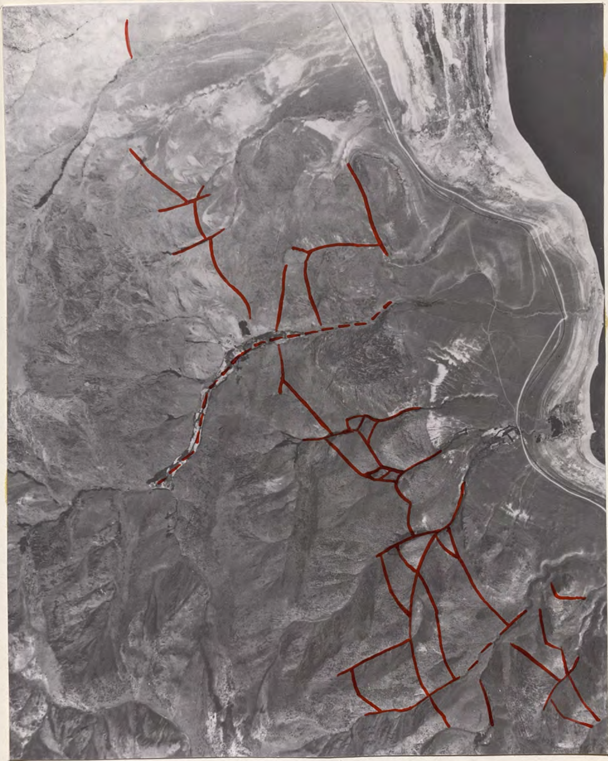
Figure 6 Fault trends in the Big Canyon area of the Low Level
