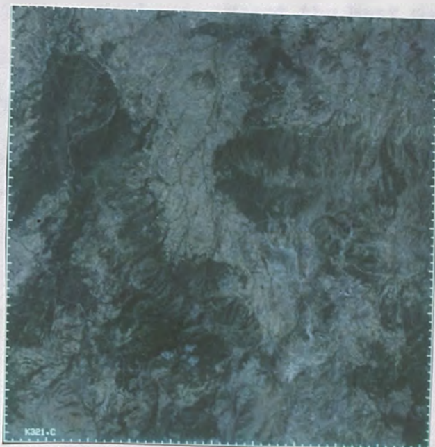
Figure 3-2. Images of study area, a) Color composite of TM bands 3, 2 and 1 (in RGB) before atmospheric correction, b) after atmospheric correction. Note bluish haze in (a).
