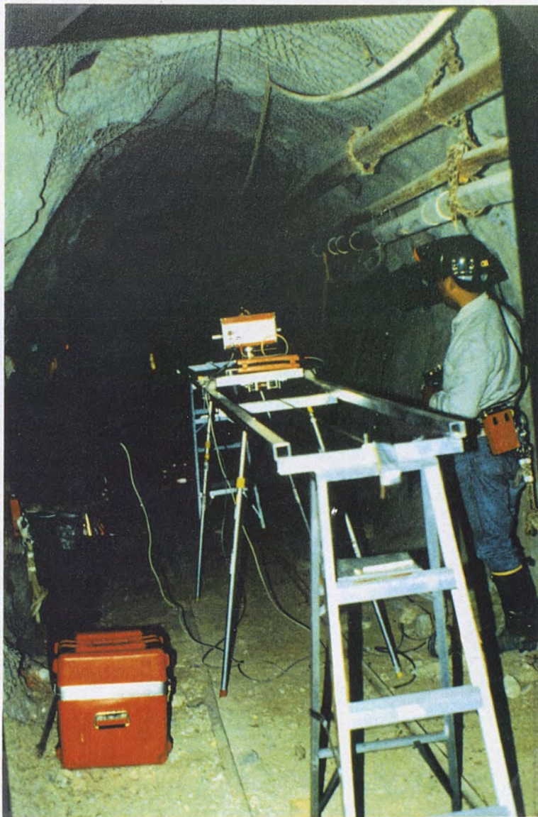
Platform and Laser Profiler in the Sunshine Mine
