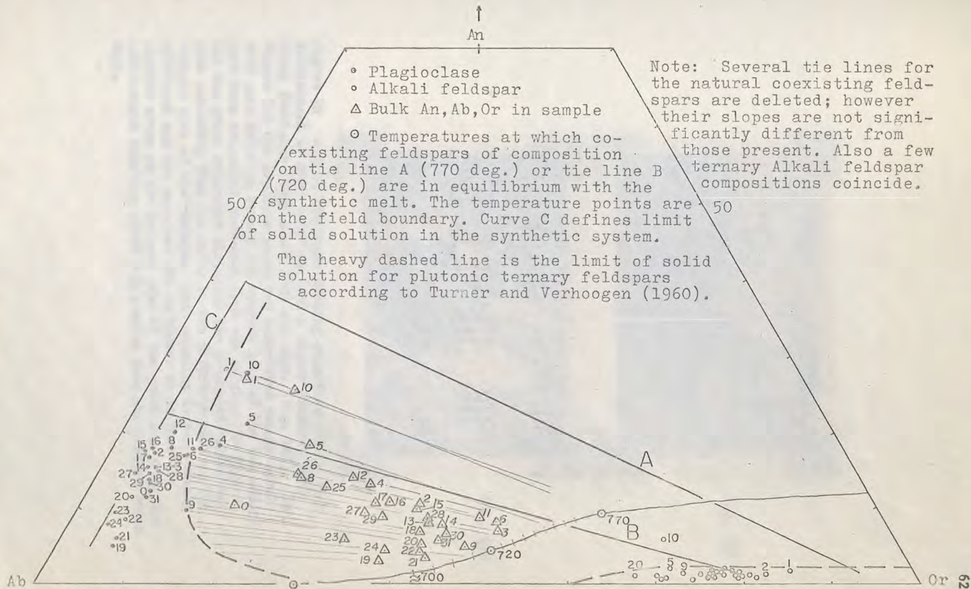
Figure 17 Coexisting feldspars from the Mineral Range, Utah, plotted on the projection of the quaternary system \text{NaAlSi}_3\text{O}_8 (Ab) - \text{KAlSi}_3\text{O}_8 (Or) - \text{CaAl}_2\text{Si}_2\text{O}_8 (An) - \text{H}_2\text{O} at 5000 bars \text{H}_2\text{O} pressure (Yoder, Stewart, and Smith, 1956-1957).
