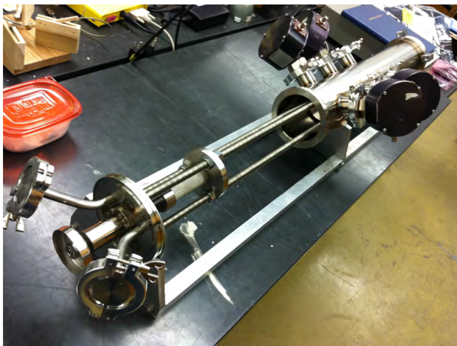
Figure 3.2: Apparatus chamber while open: The inner frame of the apparatus can be moved out of the chamber for sample loading.
