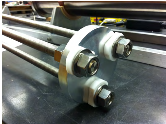
Figure 3.3: End plate to support the inner frame's weight. Three oval shaped pieces of teflon guide the frame into position in the chamber.
