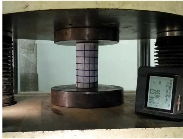
(b) Test setup of compression test
