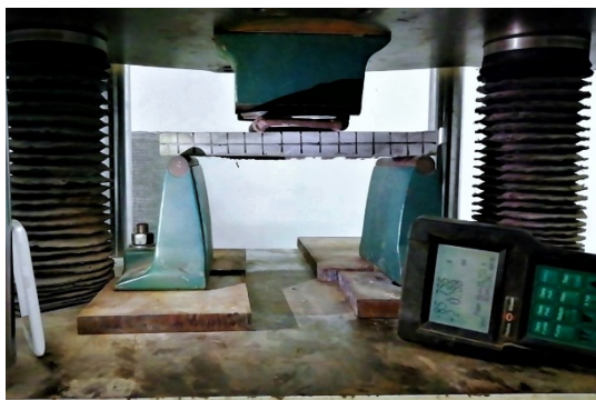
(c) Test setup of flexural strength test
