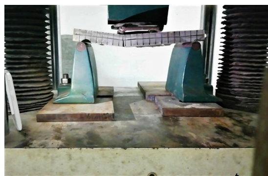
(d) Test specimen during of flexural strength test
