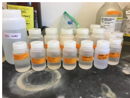
Figure 2: Pictured are some of the stock solutions made from the PFAS salts. These were made at a known concentration by dissolving the PFAS salts in water.
