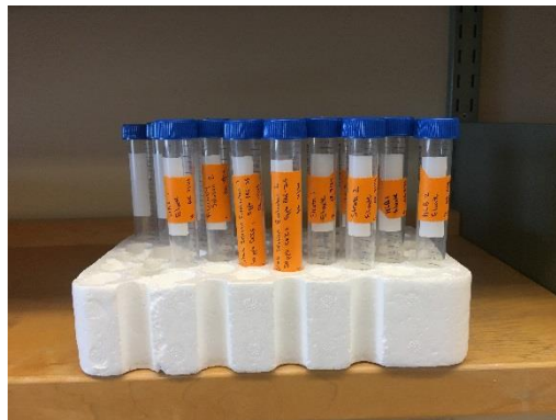
Figure 3: Samples were housed in these vials after being passed through the sorbent. These vials went under the nitrogen dryer for concentration.
