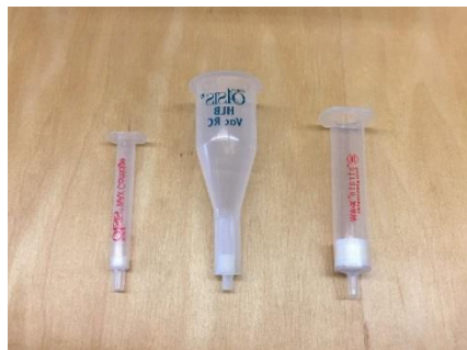
Figure 1: The sorbent material is a fine, powdery substance seen in the bottom of each plastic tube. Samples are loaded into the top of the tubes, flow through the sorbent, and exit through the narrow outlet.
