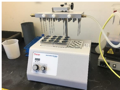
Figure 4: The sample vials are held in the metal block of the nitrogen dryer, and the needles descend into the vials just above the water surface. The dryer is connected to a nitrogen tank, and the nitrogen is gently blown out of the needles at the surface of the sample to speed evaporation.
