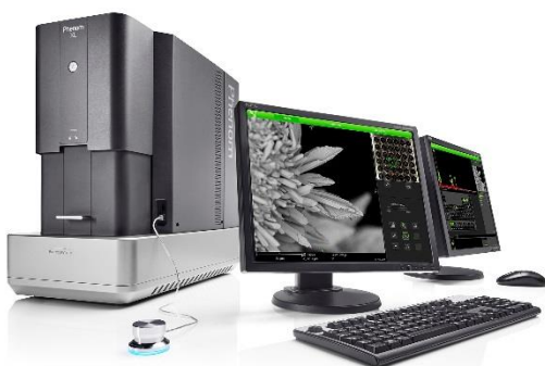
Figure 3. Shown is a scanning electron microscope. Lyophilized hydrogels were placed into the machine, and a computer was used to find the perfect angle at which to take the picture. (Photo by Phenom-World copyright 2016, Wikimedia Commons, "144243 PhenomWorld with Screenshots Tungsten.")
